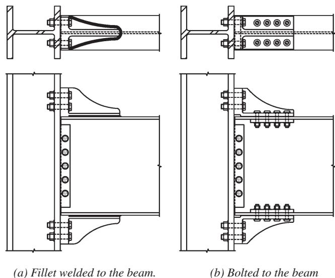
Fig. 1. Typical Kaiser bolted bracket moment-resisting connection.
