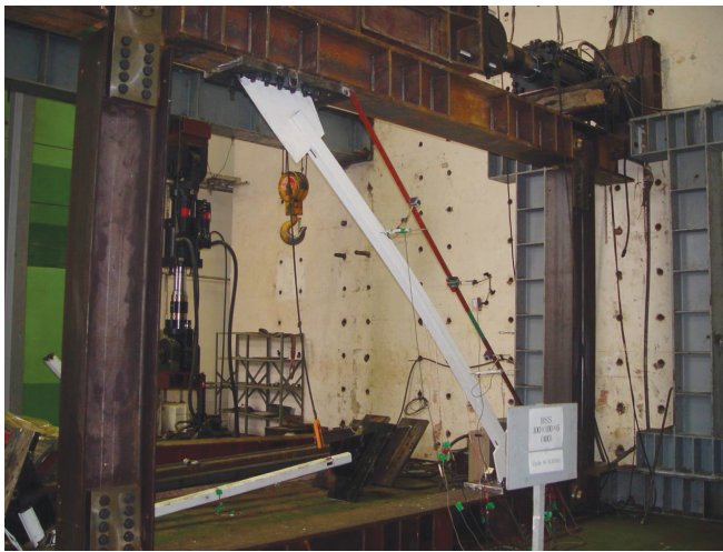
(a) Overall buckling ( -0.375\% ).
