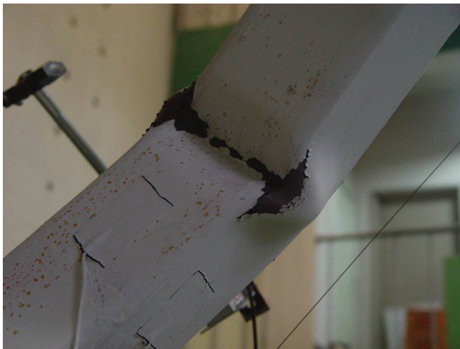
Fig. 4. Local buckling of brace 100×100×6.
