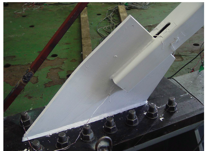
Fig. 7. Plastic zone of gusset plate.
