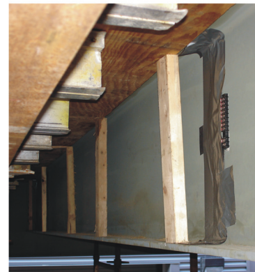
(c) Gauge installation showing form shore installed on top of gauge at this location.
