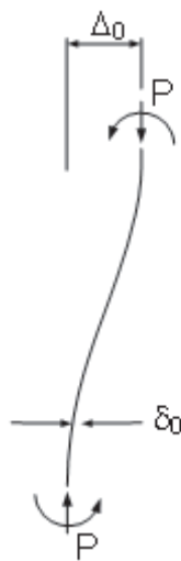
Fig. 1. Column flexure due to the axial load, P , acting through imperfections \delta_0 (out-of-straightness) and \Delta_0 (out-of-plumbness).
