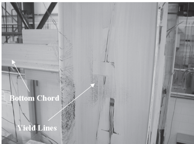
Fig. 11. Plastic hinge formation on the column.
