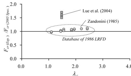
Fig. 4. Strength correlation of built-up members with welded or pretensioned bolted connectors (double channels back-to-back).
