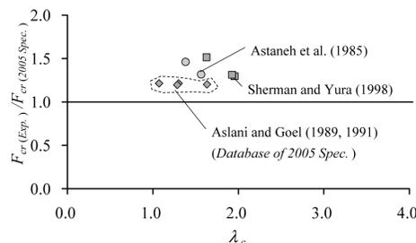
Fig. 6. Strength correlation of built-up members with welded or pretensioned bolted connectors (double angles back-to-back).
