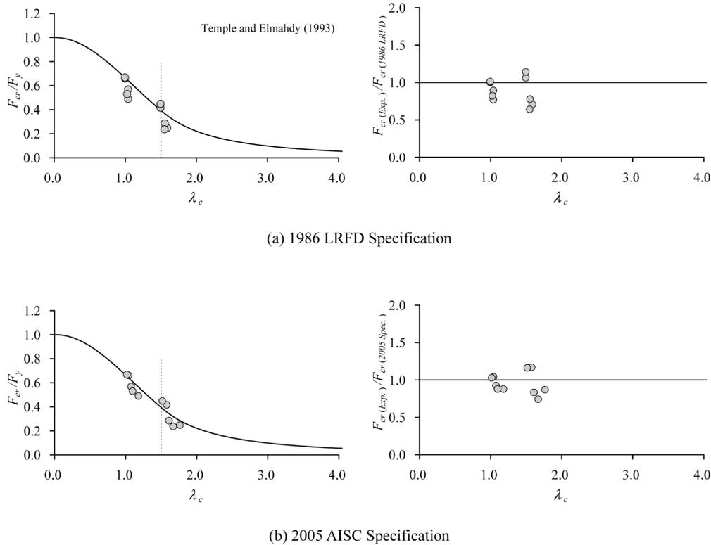
Fig. 8. Strength correlation of built-up members with welded or pretensioned bolted connectors (rectangular bars).
