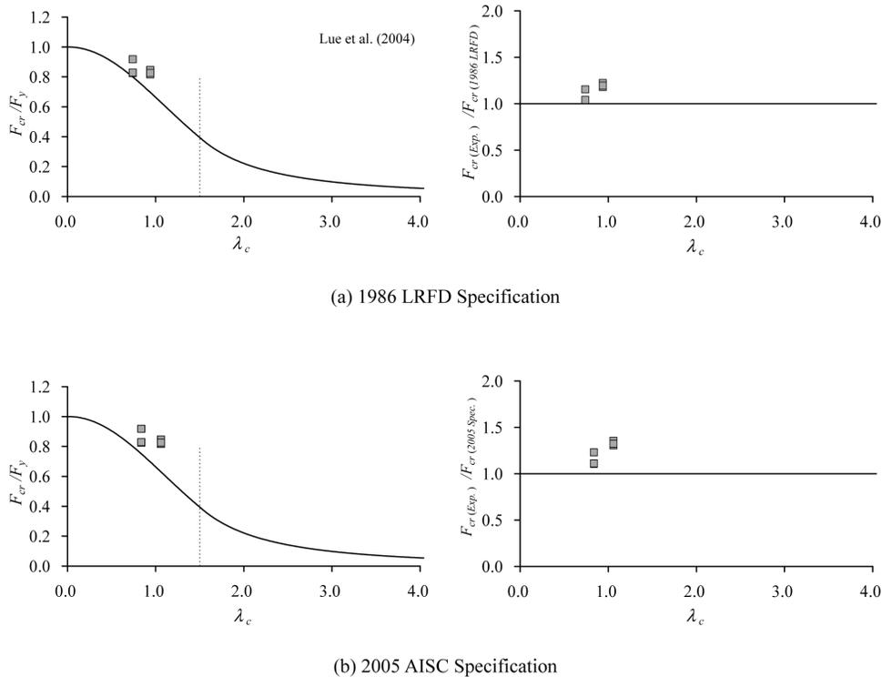
Fig. 5. Strength correlation of built-up members with welded or pretensioned bolted connectors (double channels toe-to-toe).
