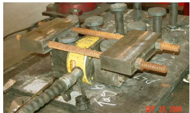
Fig. 6. Quality control test conducted by a portable hydraulic jacking system.
