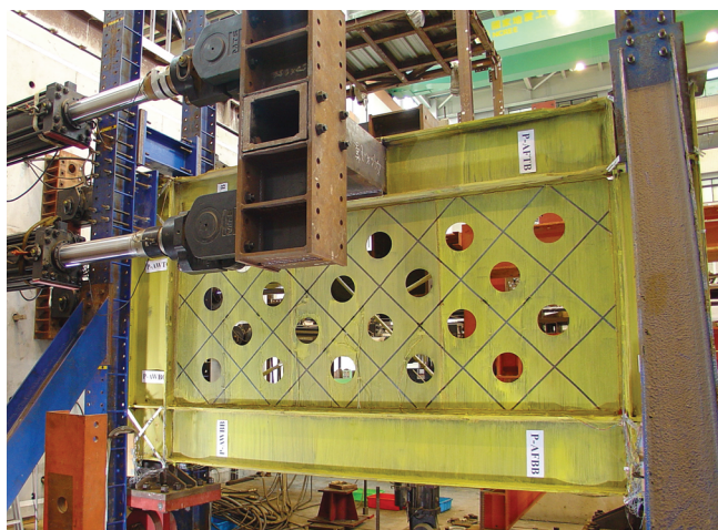
Fig. 9. Perforated panel specimen (P) before testing.
