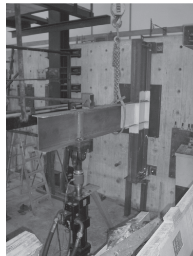
Fig. 1. Beam-column test setup.
