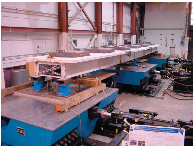
Fig. 1. Bridge model with X-brace end cross frames.
