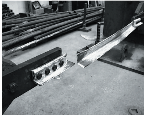
Fig. 13. Fracture of single-angle specimen with thickened bolted connection.
