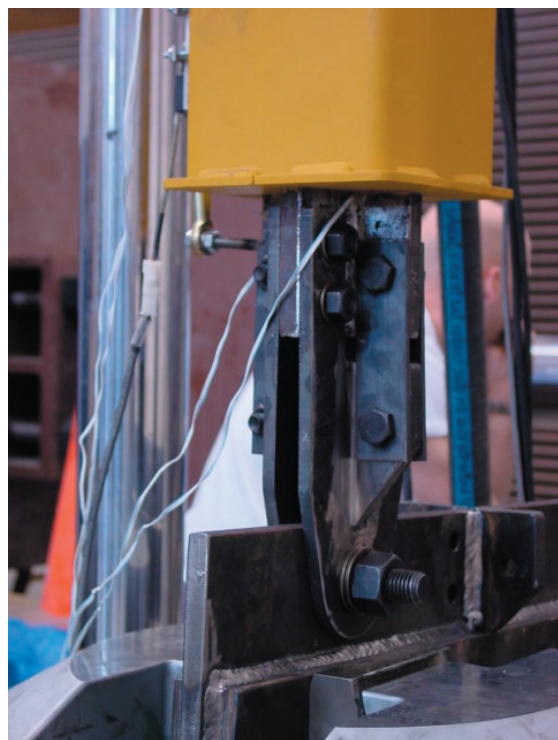
Fig. 5. Buckling-restrained brace with pinned-end connections.
