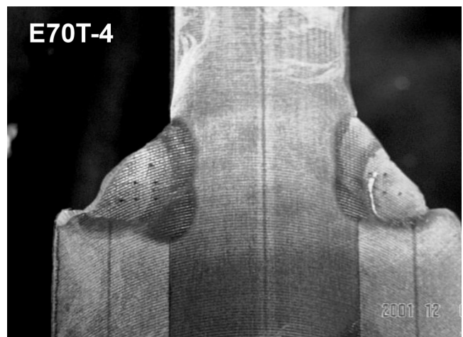
Fig. 2. Root Penetration and Extent of Fusion (12.7 mm welds shown).
