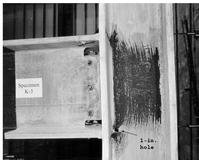
Fig. 4. Panel zone yielding pattern of specimen K3 (3% drift).
