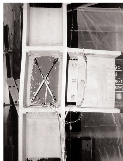
Fig. 10. Specimen K4 column kinking at 5 percent drift.
