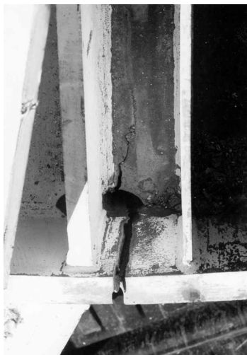
Fig. 14. Bottom flange fracture of BU30.
