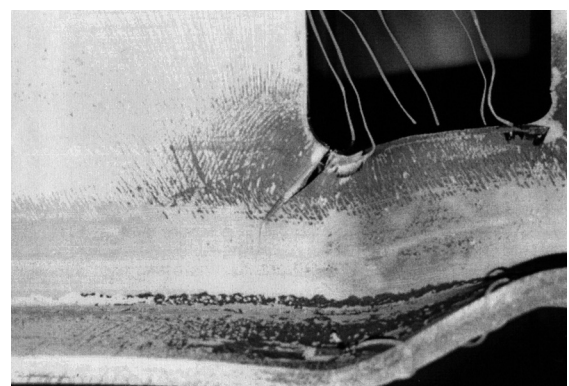
Fig. 16. Crack at opening corner (Specimen B3).
