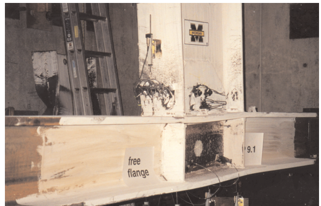
Fig. 11. Panel zone deformation and column kink in a weak panel zone Free Flange connection specimen (FF-2).
