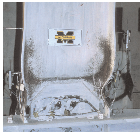
Fig. 12. Beam yielding and buckling in a strong panel zone Free Flange connection specimen (FF-3). Note that the panel zone shows no signs of yielding.
