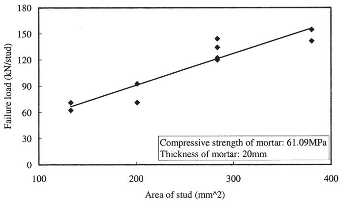
Fig. 13. Ultimate strength of the shear connection versus stud area.
