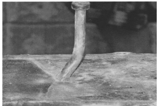
*Fig. 8. Deformed shape of the stud connector.*
