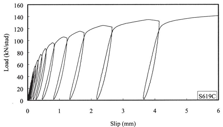
Fig. 9. Load-slip curve of the stud.
