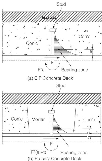
Fig. 5. Behavior of shear connection.
