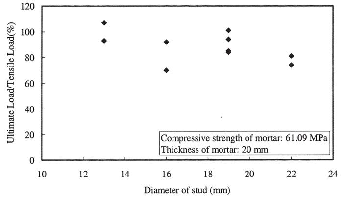
Fig. 14. Ratios of shear connection ultimate strength to tensile strength versus stud diameter.
