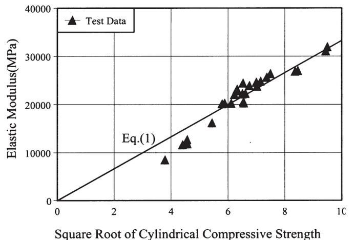
Fig. 4. Relationship between elastic modulus and compressive strength of mortar.
