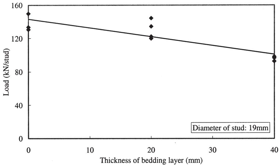
Fig. 15. Ultimate strength of the shear connection versus thickness of the bedding layer.
