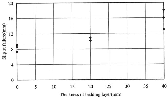
Fig. 11. Slip capacity of the shear connection versus thickness of bedding layer.
