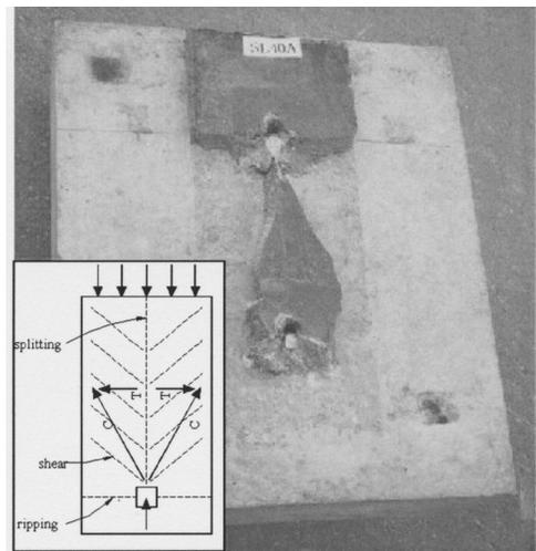
Fig. 7. Crack pattern in bedding layer.
