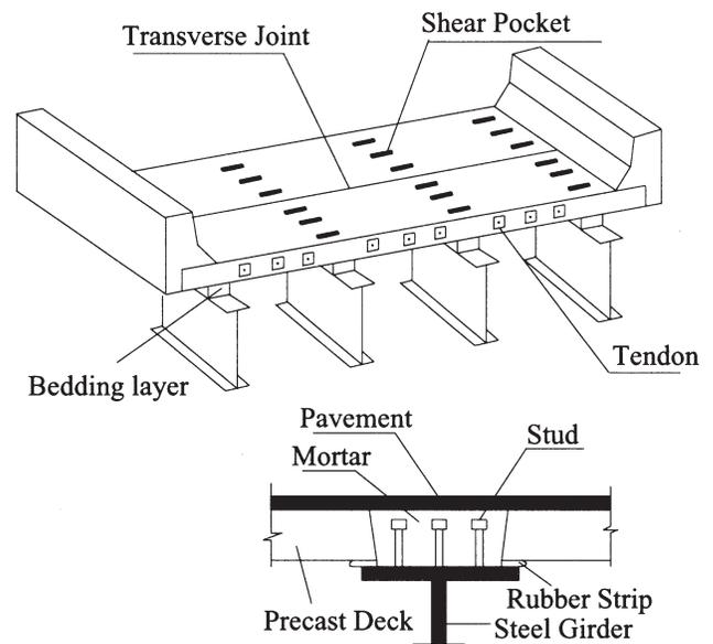
Fig. 1. Shear connection detail in full-depth precast deck.
