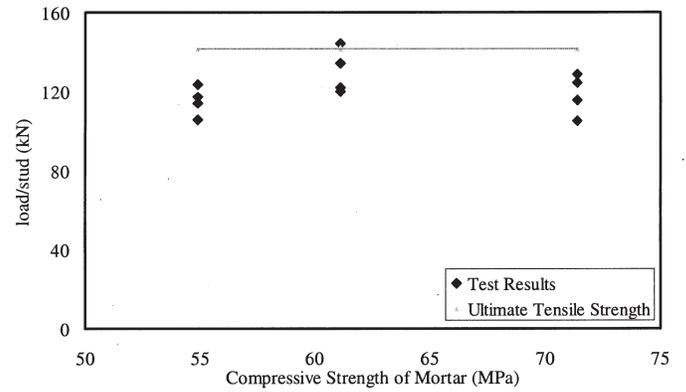
Fig. 12. Ultimate strength of the shear connection versus compressive strength of mortar.
