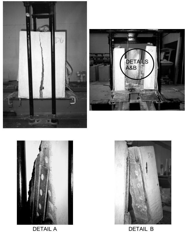
Fig. 6. Typical splitting failure (specimens without slab reinforcement).
