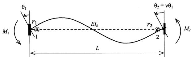
Fig. 4. End rotation of partially restrained beam.
