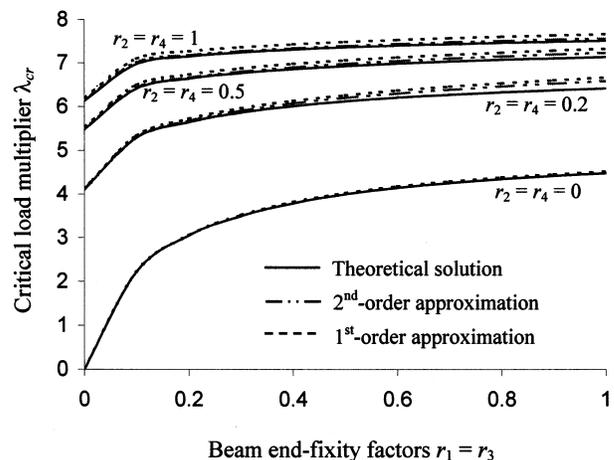
Fig. 15. Example 2:  $\lambda_{cr}$  of frame with different values of  $r$  for beams.
