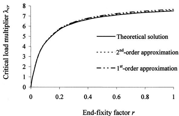
Fig. 13. Example 2:  $\lambda_{cr}$  of frame with equal value of  $r$  for beams.
