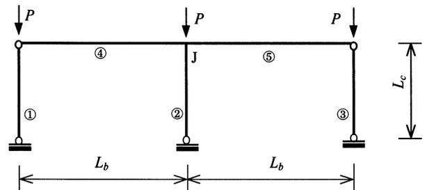
Fig. 11. Example 1: Lean-on column frame.
