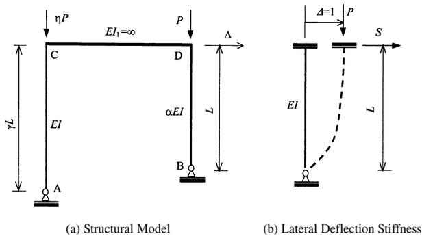
Fig. 1. Simple frame and the associated lateral buckling model.
