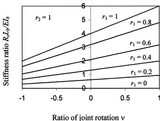
Fig. 7. Relationship between restraining stiffness and ratio of joint rotation.
