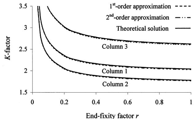
Fig. 14. Example 2:  $K$  factors associated with equal value of  $r$  for beams.
