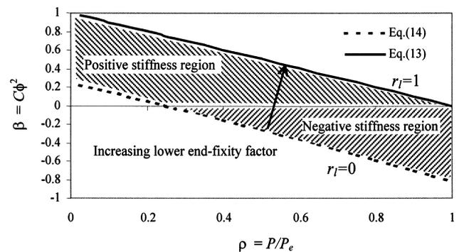
Fig. 9. Relationship between modification factor  $\beta$  and load ratio  $\rho$ .
