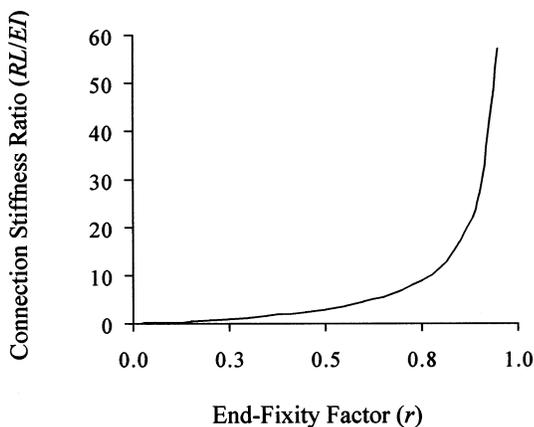
Fig. 6. Relationship between connection stiffness and end-fixity factor.
