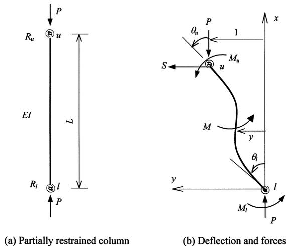
Fig. 8. Analytical model of partially restrained column.
