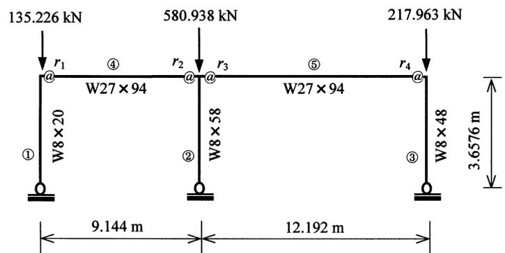
Fig. 12. Example 2: Two bays and one story frame.
