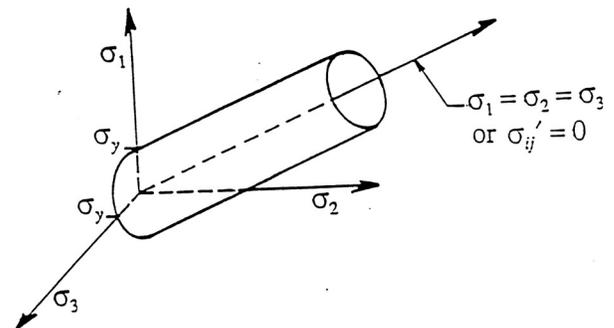
Fig. 2. Von-Mises Yield Criterion in principal stress space.
