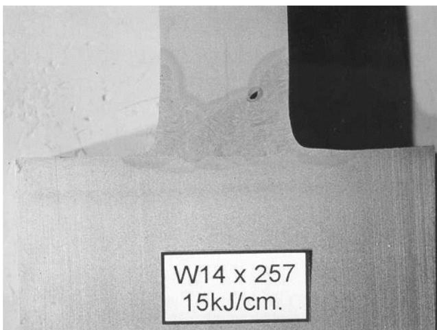
Fig. 4. Typical weld macrosection.
