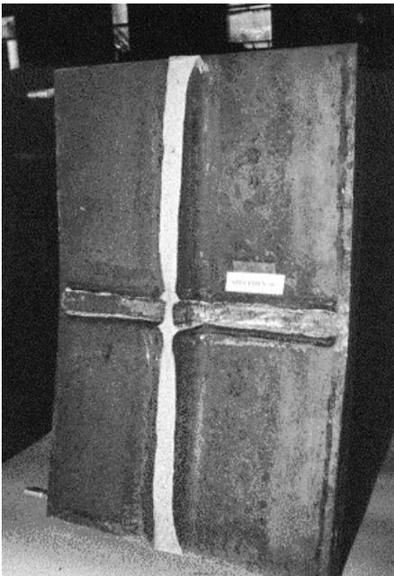
Fig. 7. Continuity plate and web failure for specimen 6. (Note, the fractured web is vertical in this photograph, and the remains of the fillet welds can be seen horizontally in the middle of the plate.)
