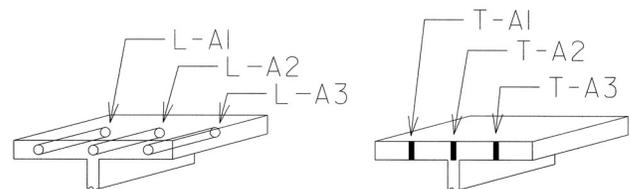
Fig. 1. Locations of uniaxial tensile test specimens.
