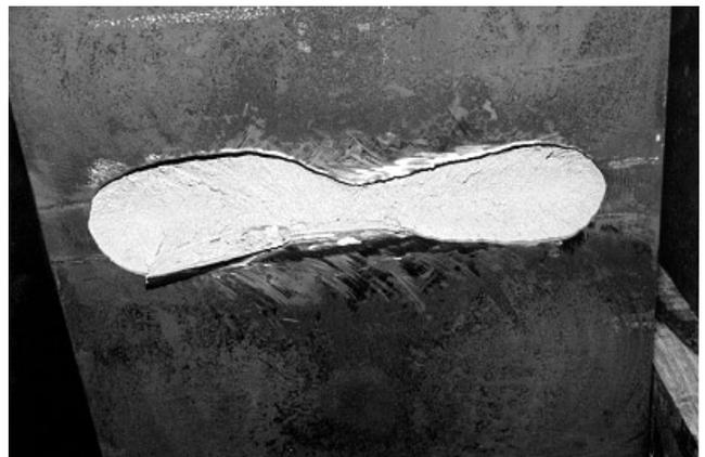
Fig. 8. View of divot-type fracture of column flange in specimen with no continuity plates. (Note, this view shows the brittle fracture on the surface of the column flange where the pull plate was. Chevron patterns are apparent on the fracture surface and point back toward the center of the flange, an indication of the origin of the fracture.)
