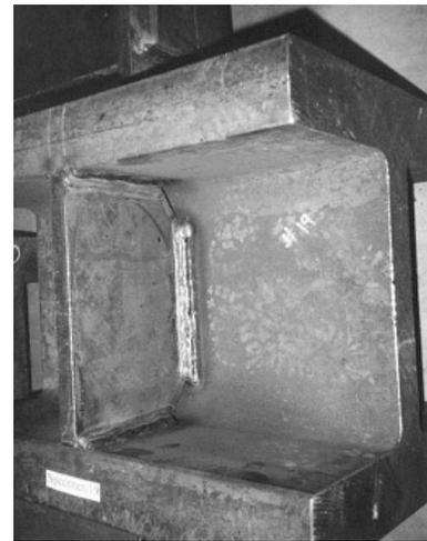
5a) specimen with groove-welded continuity plates and AISC recommended cutouts in the continuity plates (AISC, 1997)
