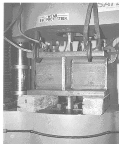
5b) specimen with fillet welded continuity plates and inadequate cutouts in the continuity plates showing pull-plate failure in top pull plate
