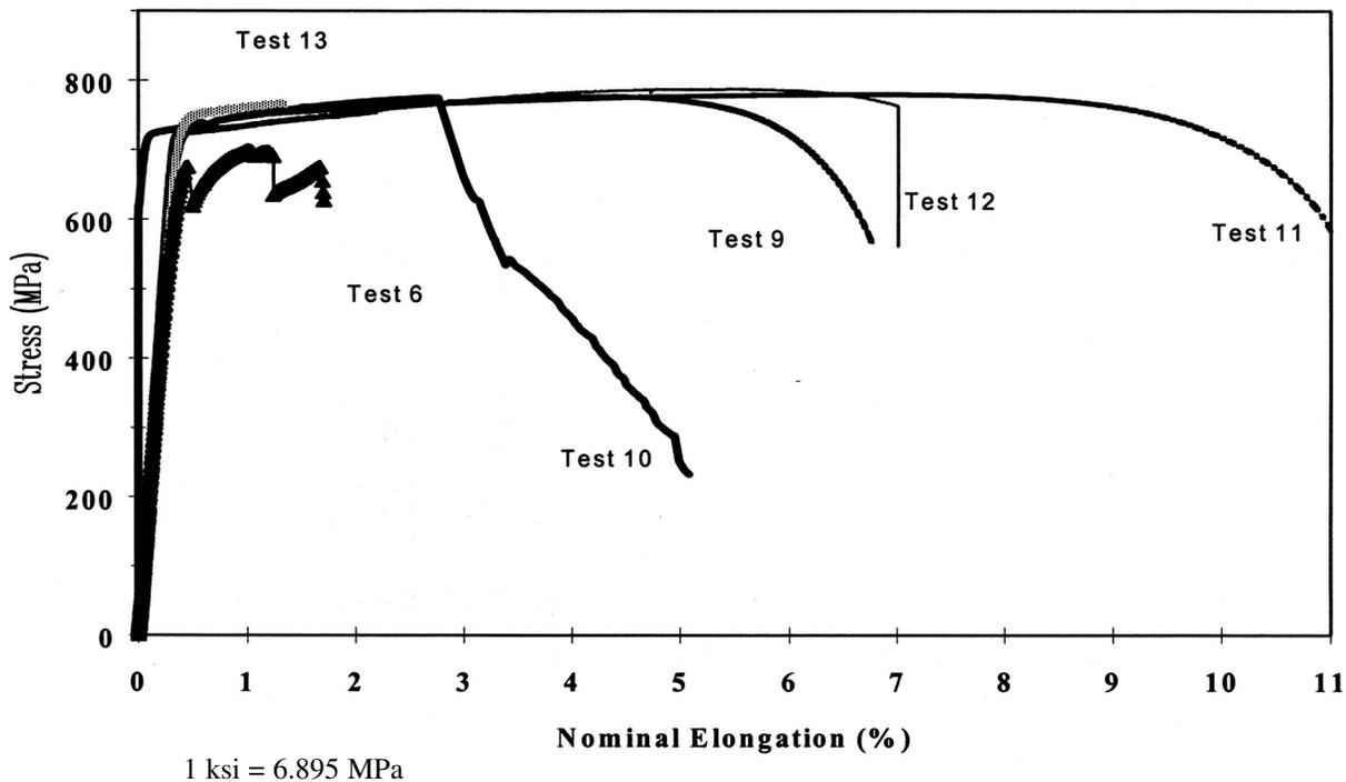
Fig. 6. Nominal pull-plate stress vs. elongation curves for six specimens with 305 mm (12 inch) pull plates.
