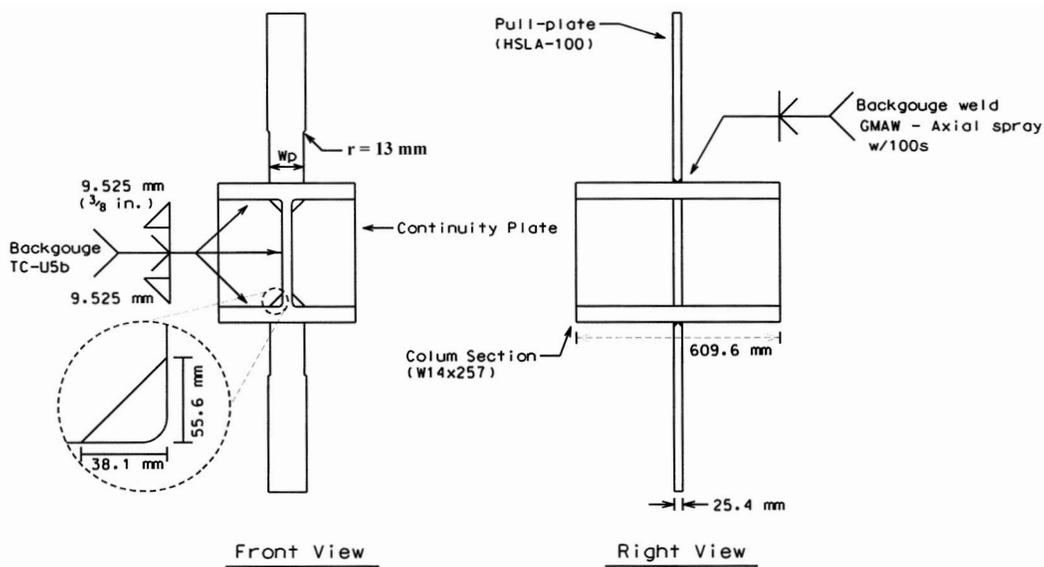
Fig. 3. Basic configuration of tee-joint test specimen (1 inch = 25 mm).
