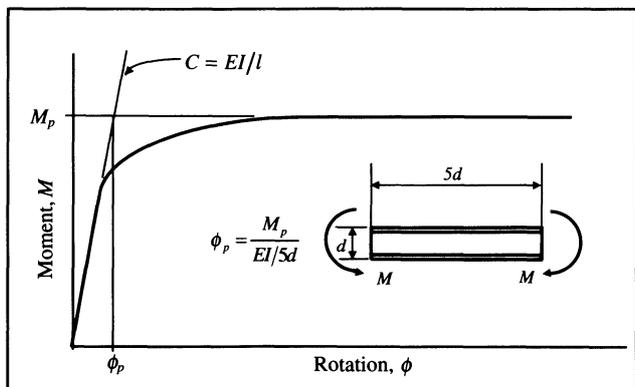
Fig. 2(b). Beam Moment-Rotation Curve
