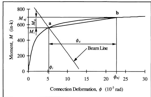
Fig. 10(a). Loading After Initial Deformation
