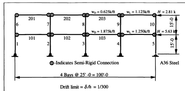
Fig. 11. Semi-Rigid Unbraced Frame Example<sup>13</sup>
