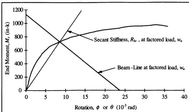
Fig. 6. Beam-Line Diagram with  $M-\phi$  Curve<sup>10</sup>
