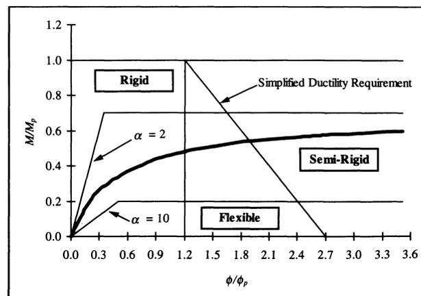
Fig. 2(a). Non-Dimensional Classification of Connections<sup>6</sup>
