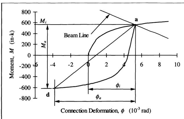
Fig. 10(c). Unloading After Initial Deformation ( $|M_a| > |M_i|$ )
