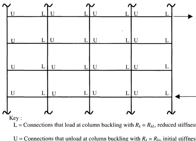
Fig. 5. Connection Behavior at Column Buckling in an Unbraced Frame
