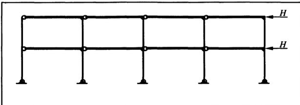
Fig. 12. Unbraced Frame with Wind Load
