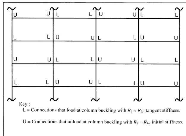
Fig. 3. Connection Behavior at Column Buckling in a Braced Frame
