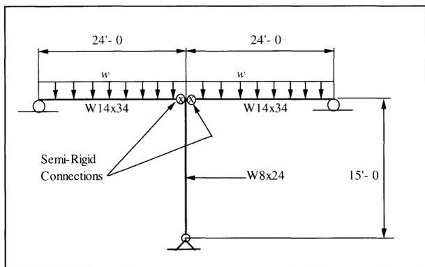
Fig. 4(a). Unbraced “Tee”—Load Sequence 1
