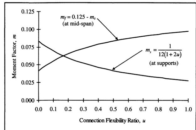
Fig. 7. Optimum Connection Flexibility (Symmetrically Supported Beam)
