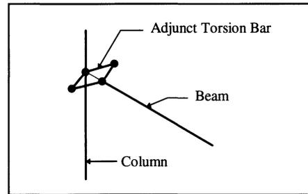
Fig. 9. Connection Model Using Torsion Elements
