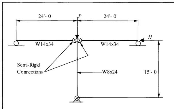
Fig. 4(b). Unbraced “Tee”—Load Sequence 2
