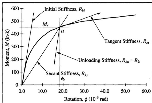
Fig. 1. Moment vs. Rotation for a Flush End-Plate Connection<sup>24</sup>
