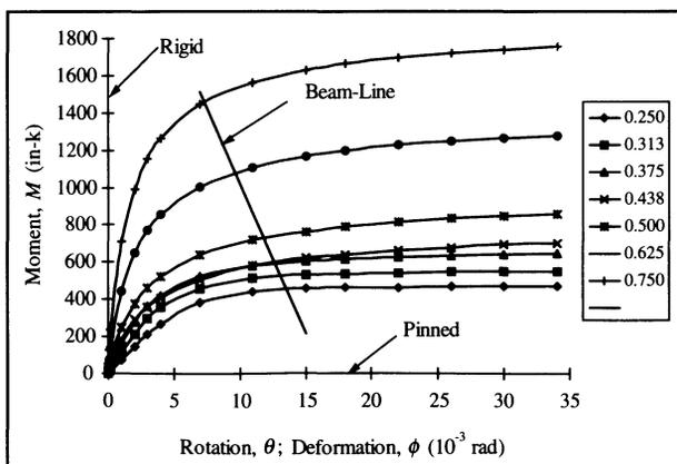
Fig. 8. Influence of Connection Behavior on Beam Response<sup>11</sup>
