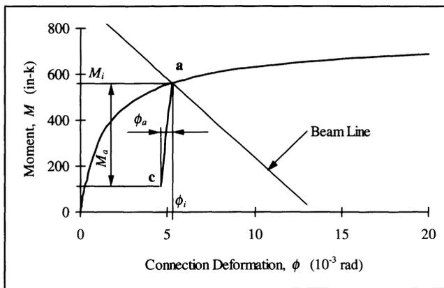
Fig. 10(b). Unloading After Initial Deformation ( $|M_a| < |M_i|$ )
