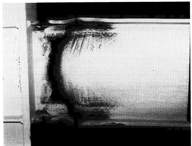
Fig. 12. Specimen DB4 at end of test ( $\theta_p = 0.037$  radian).
