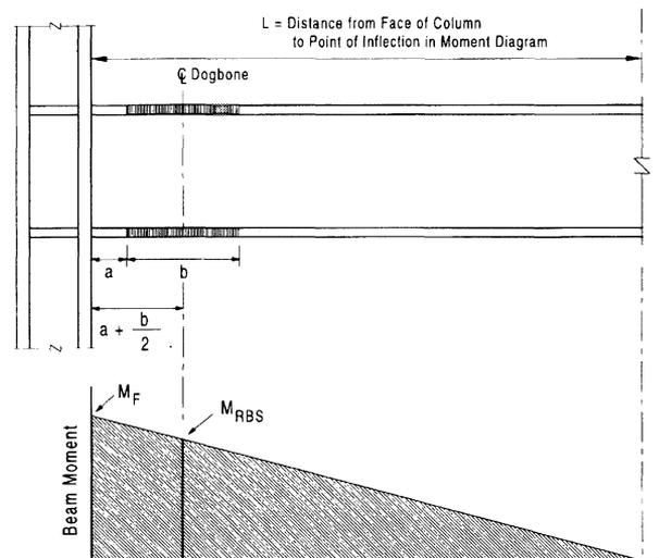
Fig. 14. Assumed moment diagram for design of dogbone cutout.
