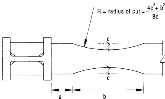
Fig. 13. Geometry of radius cut dogbone.
