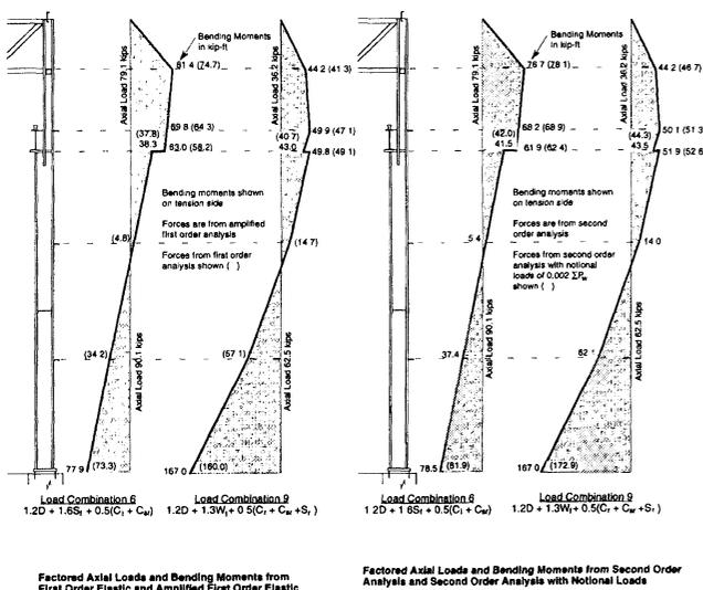
Fig. 5. Factored axial loads and bending moments for four methods of analysis.
