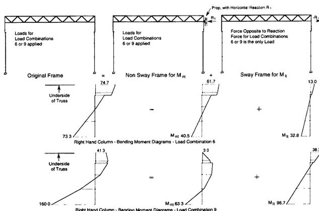
Fig. 2. Frame models for  $M_{nt}$  and  $M_{lr}$ .
