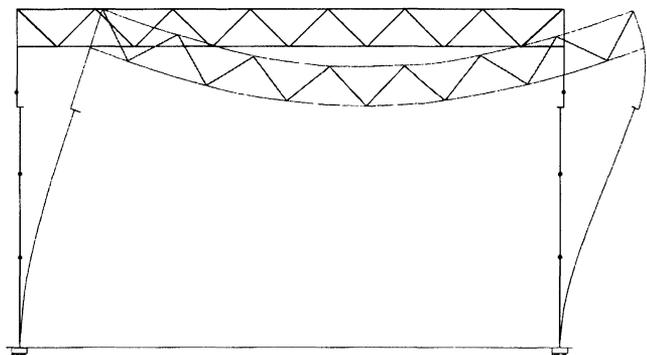
Fig. 6. Computer model frame showing typical exaggerated deflected shape.
