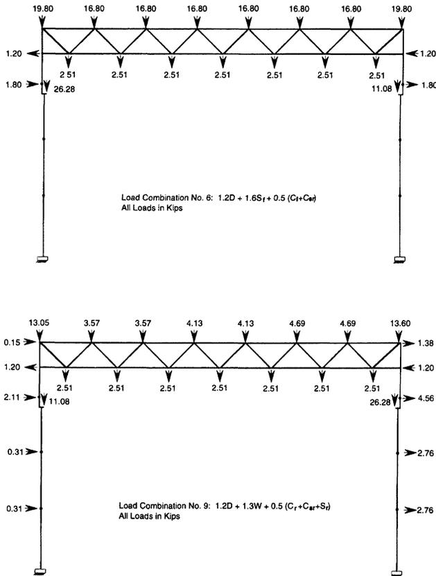
Fig. 3. Governing factored load combinations for stepped column.
