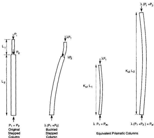
Fig. 7. Equivalent lengths for the two segments of a fixed-slider column.
