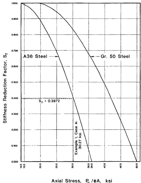
Fig. 5. Stiffness reduction curves.
