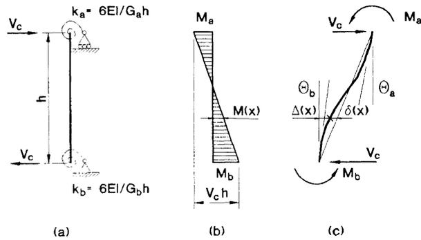
Fig. 2. First order deflection of a stability column.
