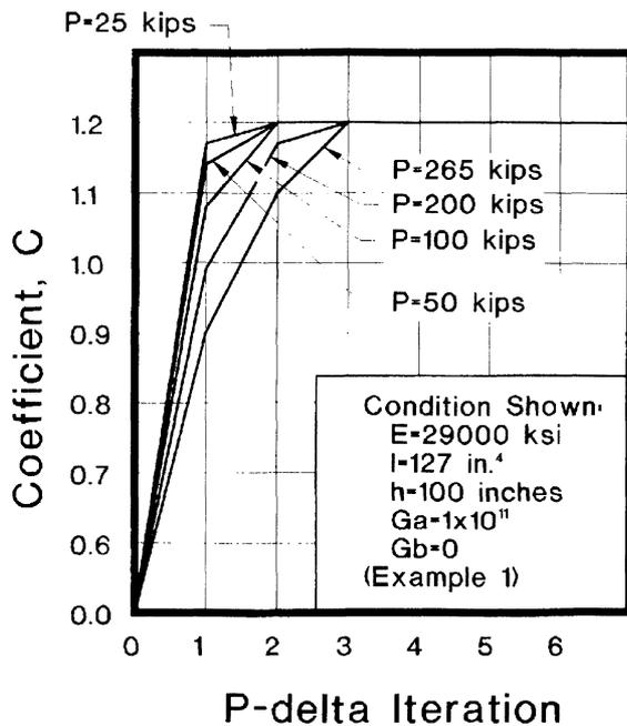
Fig. 4. Effect of  $P$ -delta iterations on second order deflections.
