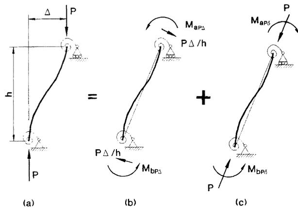
Fig. 3.  $P$ -delta effects on a stability column.
