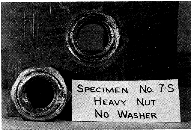
Fig. 17. Galled surface under nut torqued without hardened washer
