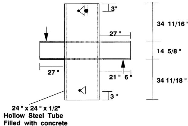
Fig. 5. General configuration of test specimen.
