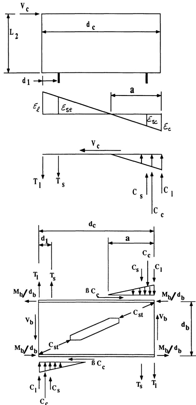
Fig. 10. FBD of the upper column and beam web within the joint area.
