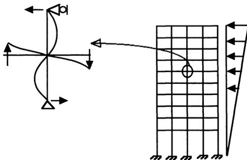
Fig. 9. Assumed forces on an interior joint in a frame subjected to lateral loads.
