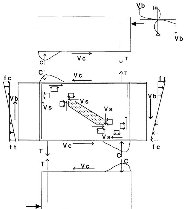
Fig. 4. Force transfer mechanism for through beam connection detail.
