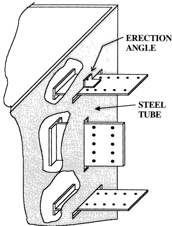
Fig. 2. Type A connection detail using embedded elements.
