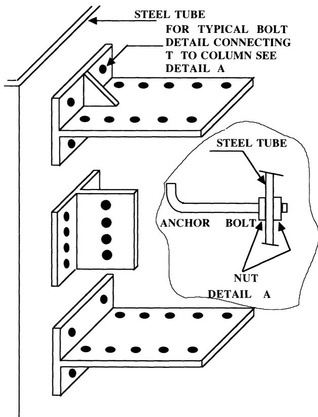
Fig. 1. Type A connection detail using anchor bolt.
