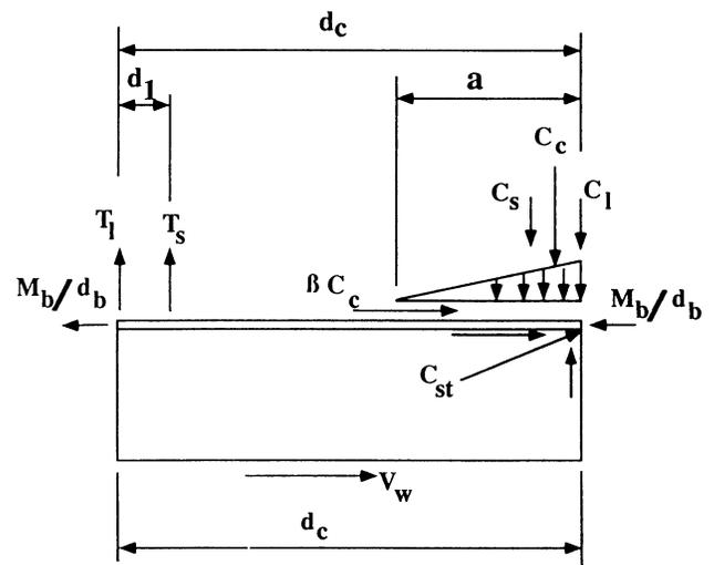
Fig. 11. FBD of the portion of the web within the joint area.
