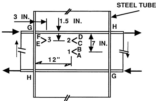
Fig. 7. Location and orientation of gages attached to beam web within the column.
