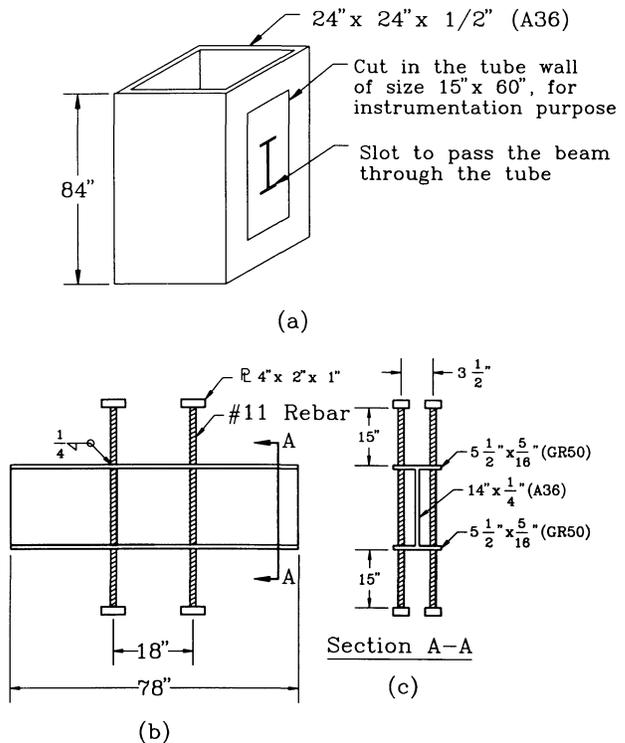
Fig. 6. Different components of the test specimen: a) hollow steel tube, b) hybrid built-up beam section, c) four #11 reinforcing bars with anchor plates welded to each end.
