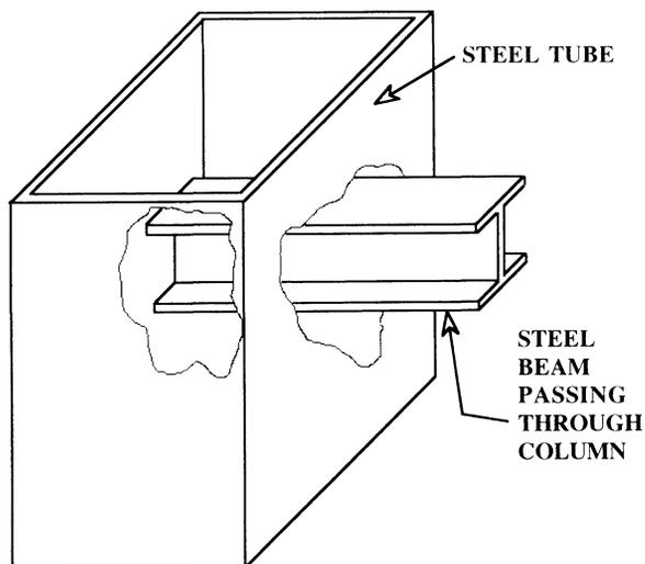
Fig. 3. Through connection detail.
