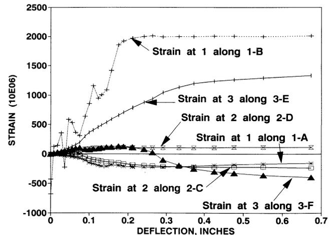
Fig. 8. Strain data from gages attached to beam web within the column.
