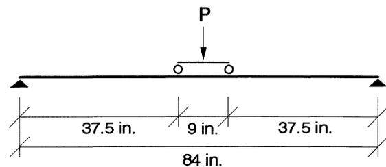
Fig. 3. Positive bending test.
