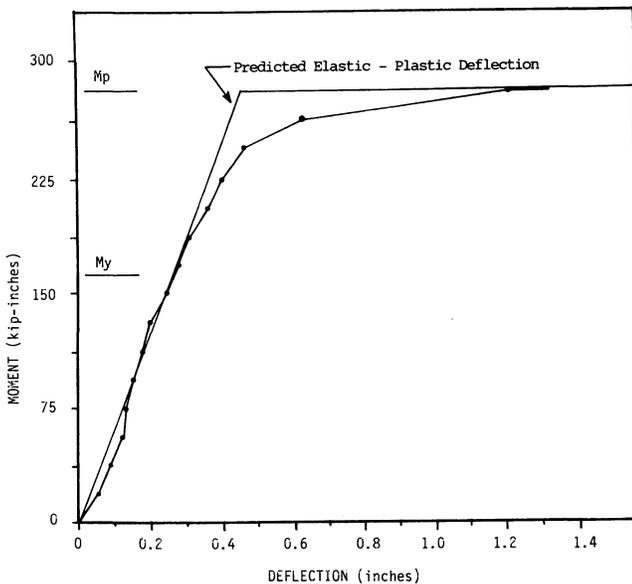
Fig. 6. Moment vs. deflection for Test 4.
