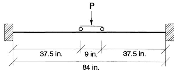
Fig. 4. Negative bending test.
