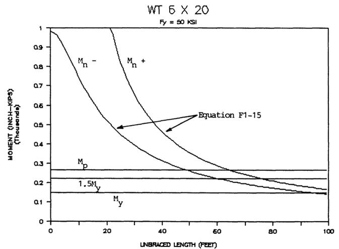
Fig. 10. Flexural strength of WT6x20,  $F_y = 50$  ksi.
