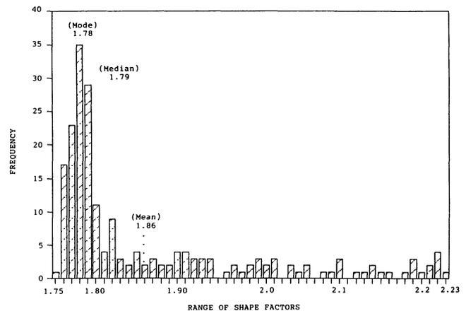
Fig. 1. Variation of shape factor for WT section.
