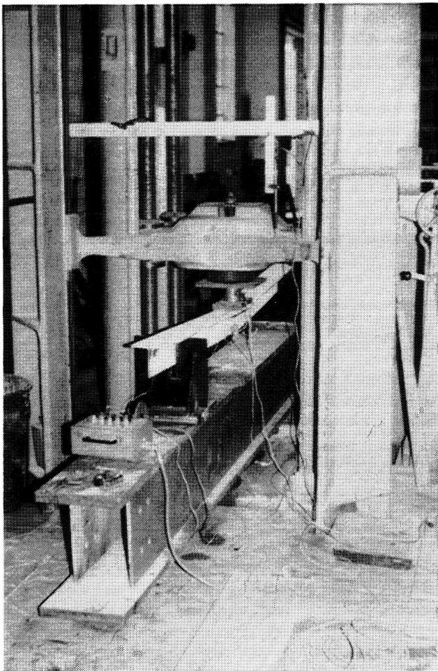
Fig. 2. Test beam in loading fixture.
