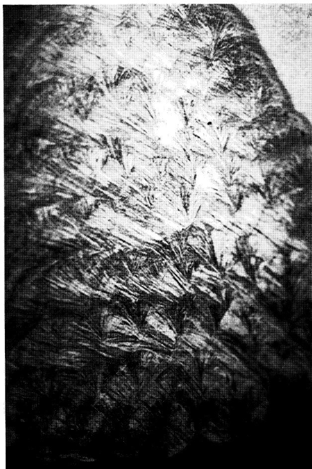
Fig. 6. Dendritic crystalline formation on a polished and etched full penetration weld on a thick flange.
