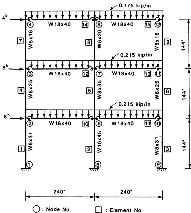
Fig. 11. Partially-restrained frame FR-4.
