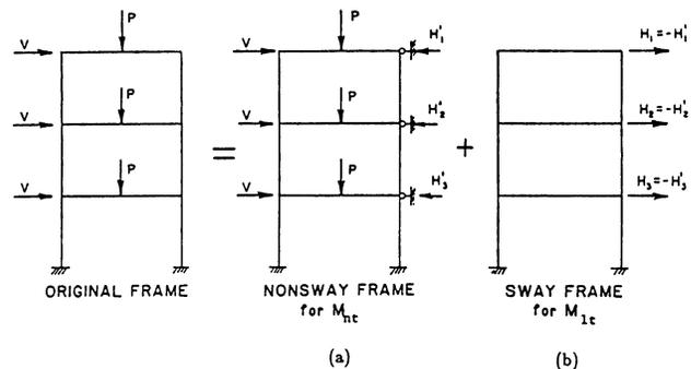
Fig. 1. Two fictional frames for determining frame moments.
