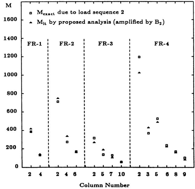
Fig. 15. Comparison of column moments due to sway loads in frames with connection III-14 of medium rigidity.
