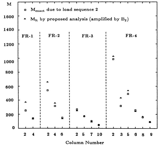
Fig. 16. Comparison of column moments due to sway loads in frames with the more rigid connection III-17.
