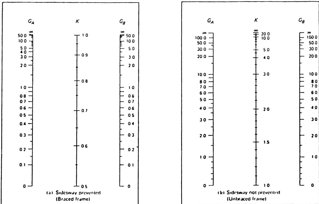
Fig. 5. Alignment charts for the determination of the effective length factor  $K$ .
