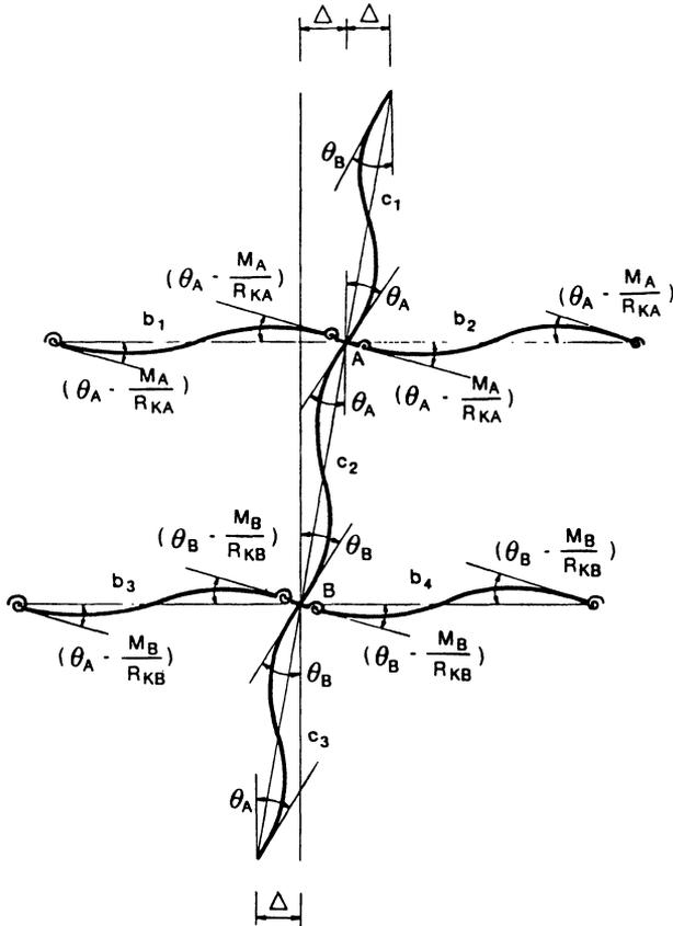
Fig. 7. Subassembly model for unbraced (sway) frame.
