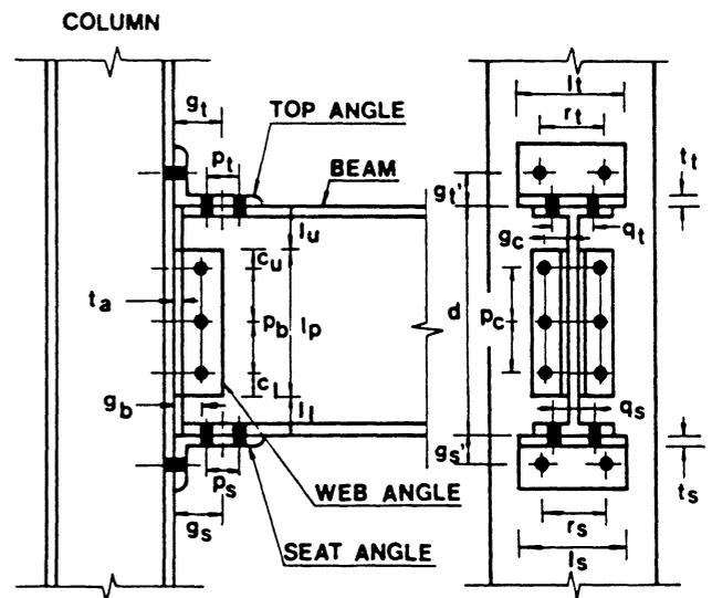
Fig. 3. Typical top- and seat-angle with double web-angle connection.
