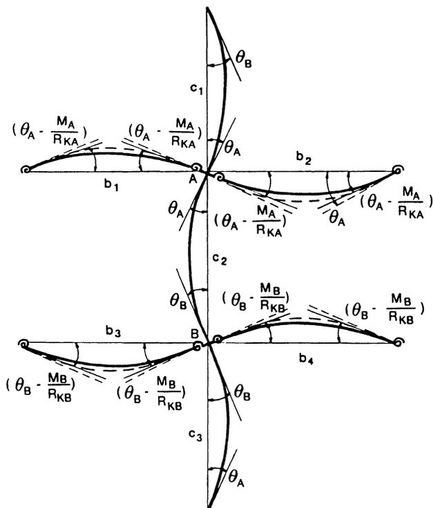
Fig. 6. Subassembly model for braced (nonsway) frame.
