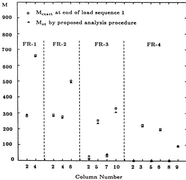
Fig. 14. Comparison of column moments due to nonsway loads in frames with the more rigid connection III-17.
