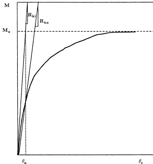
Fig. 2. Initial and modified initial stiffness for  $M_u$  calculations.
