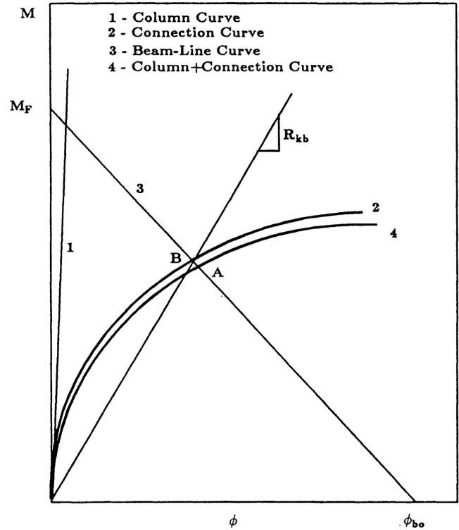
Fig. 4. Moment-rotation curves for joint components and the determination of  $R_{kb}$  for  $M_{lt}$
