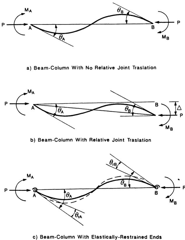
Fig. 8. Beam-column subjected to end moments.
