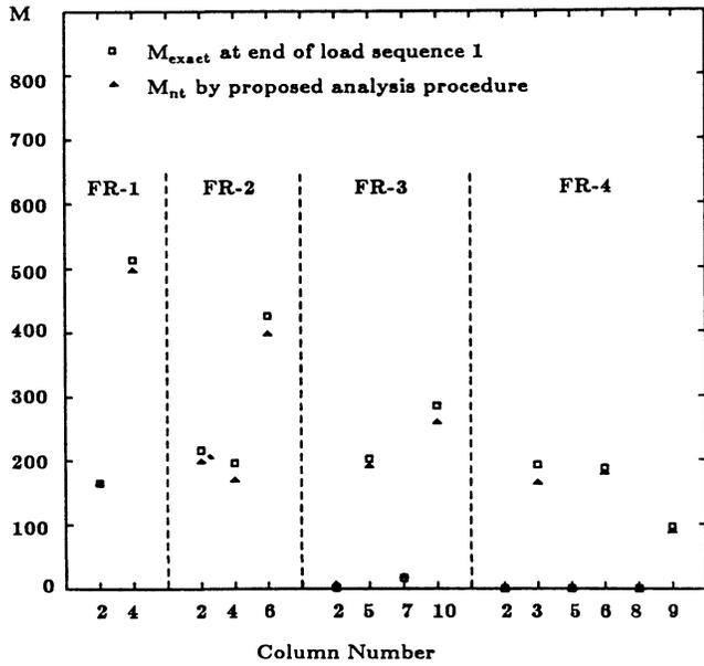
Fig. 13. Comparison of column moments due to nonsway loads in frames with connection III-14 of medium rigidity.
