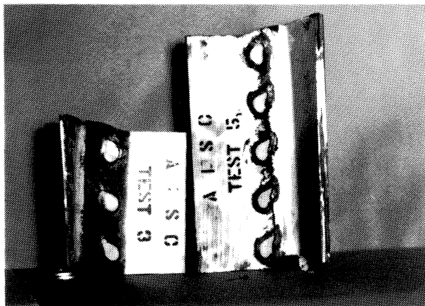
Fig. 9. Failure of Net Section of Tee Stems
