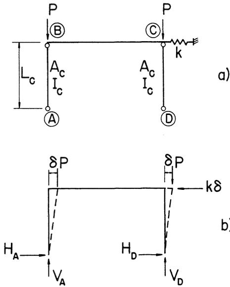
Fig. 3. Idealized bracing arrangement
