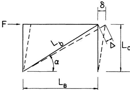
Fig. 5. Deformation of the bracing member
