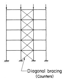
Fig. 1. Lateral stability provided by diagonal bracing
