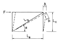
Fig. 5. Deformation of the bracing member
