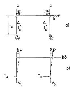
Fig. 3. Idealized bracing arrangement
