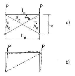
Fig. 2. Buckling of a simple braced frame
