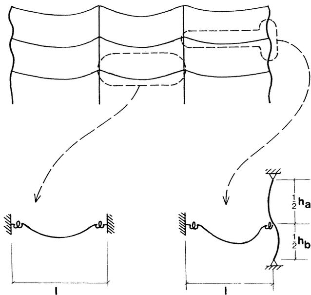
Fig. 3. Flexibly connected girder models
