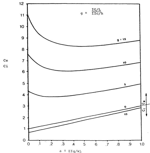
Fig. 4. Flexible end-moment coefficients
