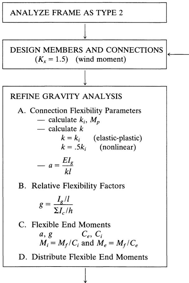
Fig. 5. Simplified PR design procedure
