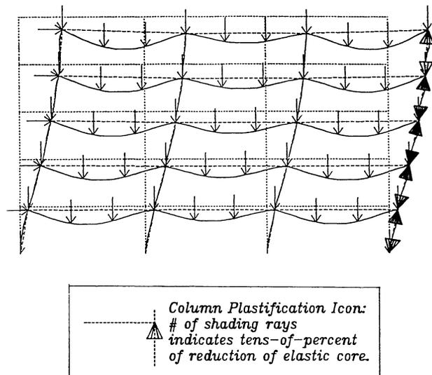
Fig. 1. Typical limit-state mode for simply connected frames
