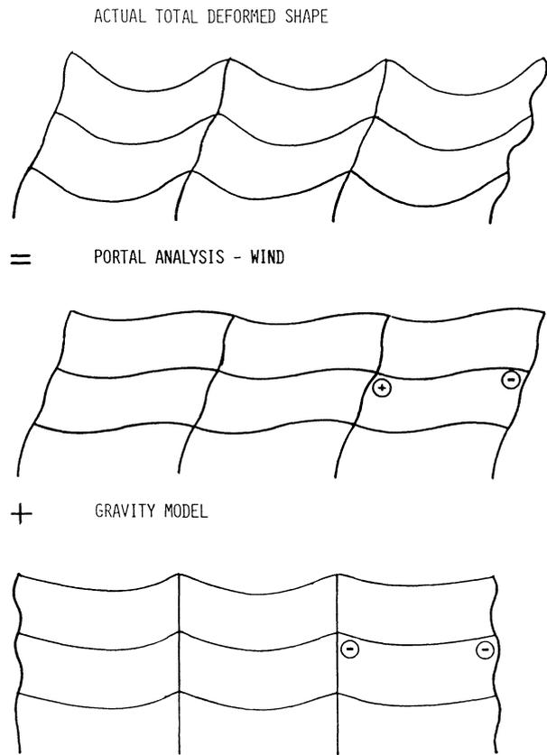
Fig. 2. Component deformed shapes
