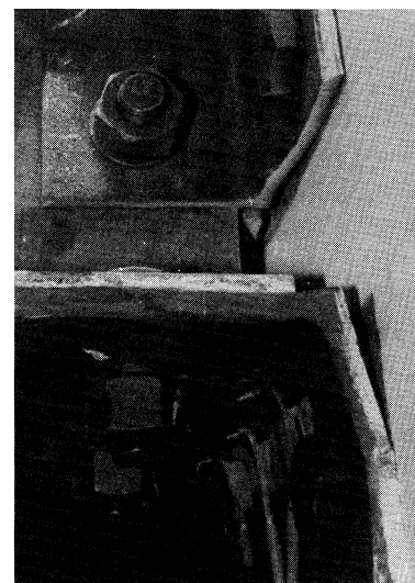
Fig. 19. Pullout of angles in tension
