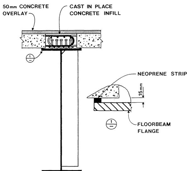
Fig. 8. Floor beam—precast deck joint
