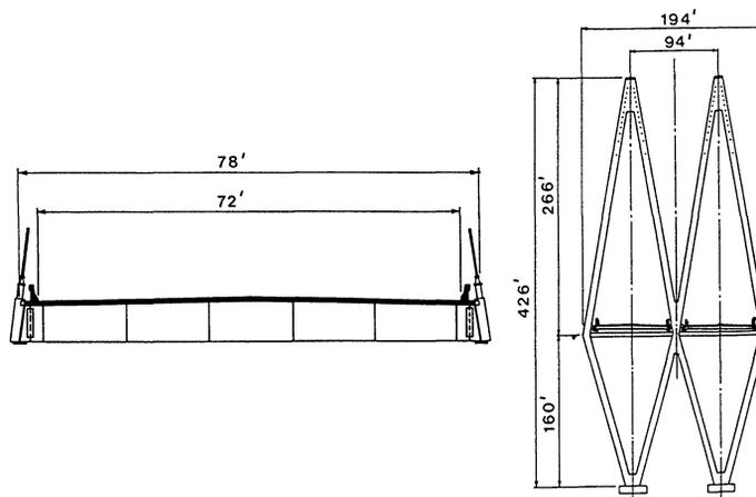
Fig. 2. Cross section—Houston Ship Channel Bridge
