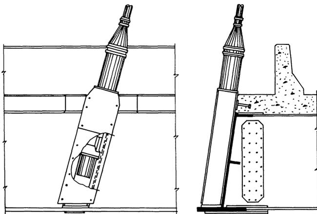
Fig. 5. Typical stay connection, Houston Ship Channel Bridge
