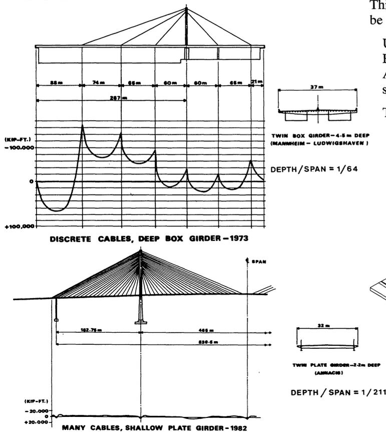
Fig. 3. Comparison of dead-load bending moments
