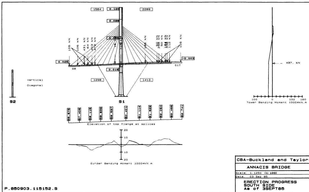
Fig. 10. Computer plot of balance analysis
