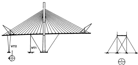
Fig. 9. Temporary restraints during erection
