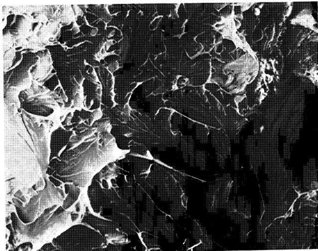
Fig. 33. Fractograph of clean fracture area in Fig. 6 @ 100x showing cleavage facets
