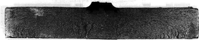
(a). Fracture surface of flange
