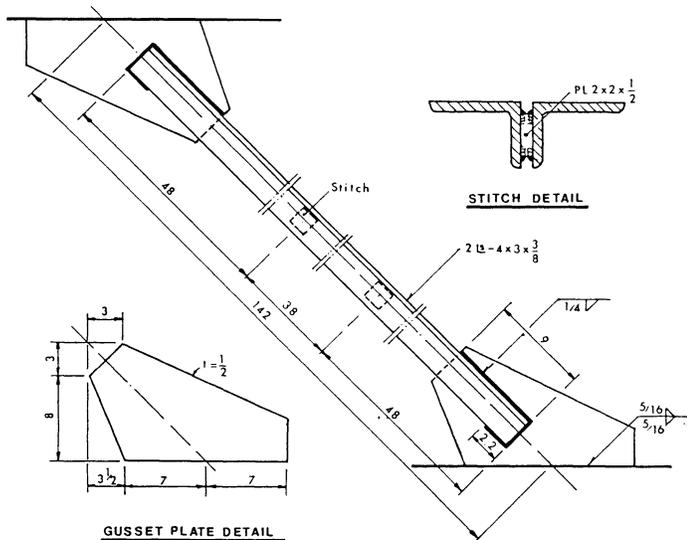
Fig. 15. Welded double angle bracing member of Example 2
