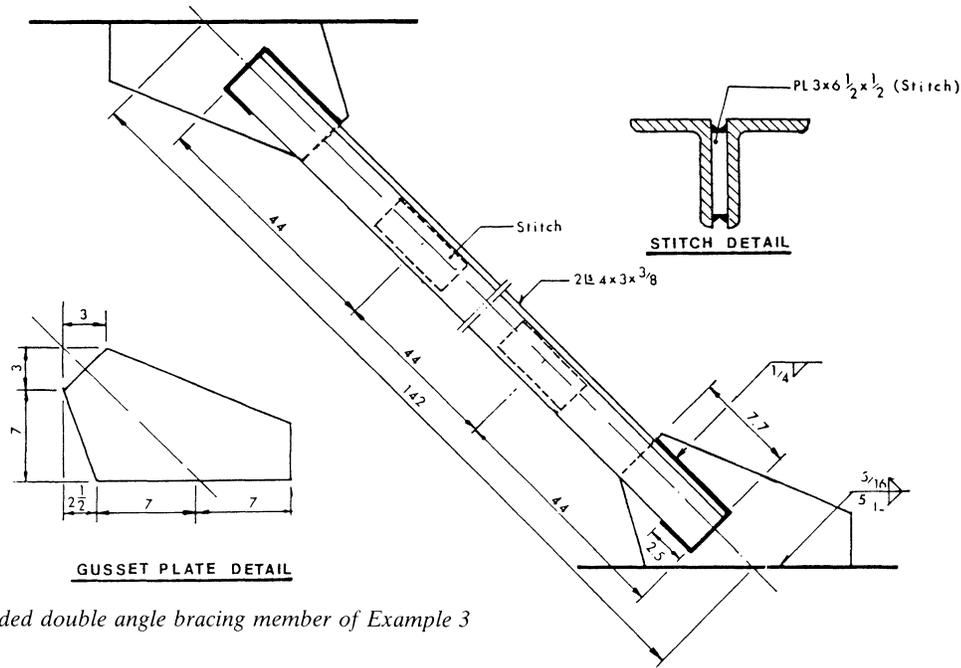
Fig. 16. Welded double angle bracing member of Example 3
