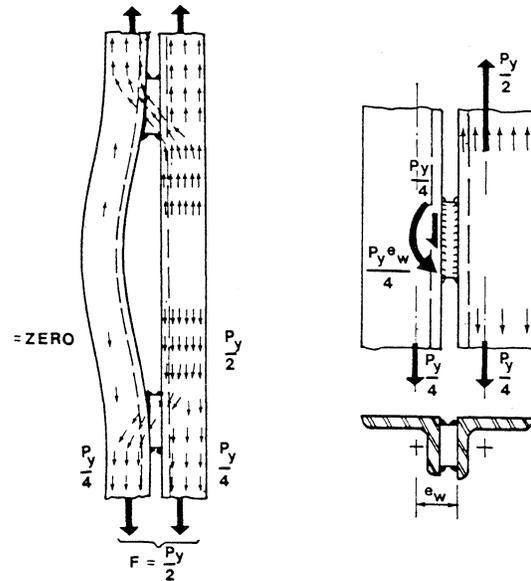
Fig. 6. Design forces for stitches in out-of-plane buckling bracings
