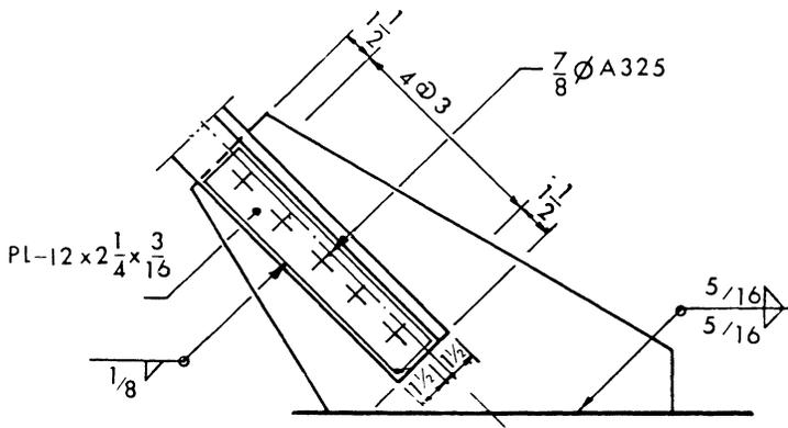
Fig. 14. Reinforced connection
