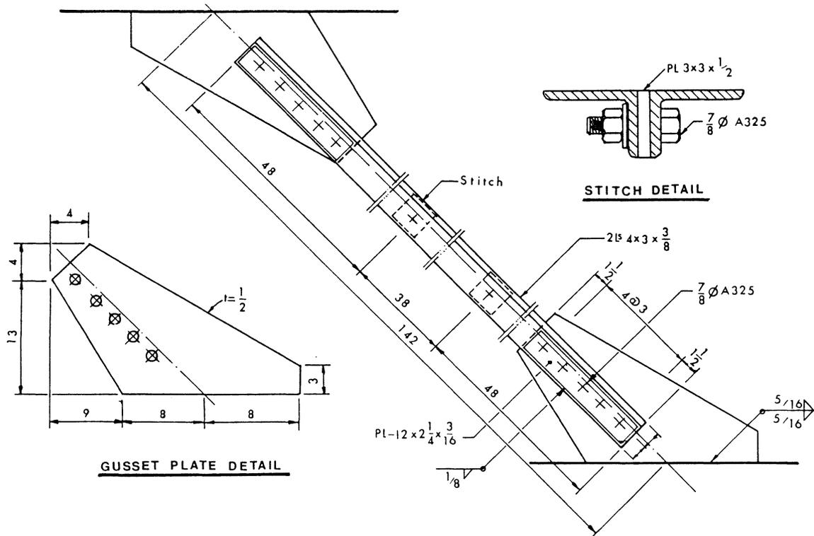
Fig. 12. Bolted double angle bracing member of Example 1
