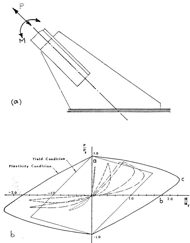
Fig. 7(a). Design forces for end connections of in-plane buckling bracings
