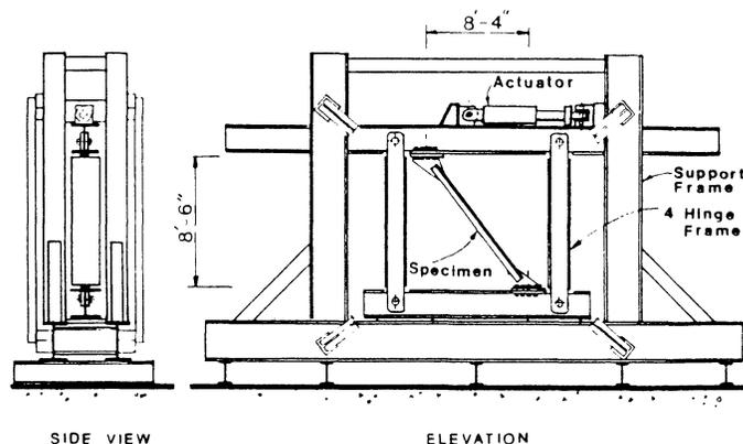
Fig. 1. Test specimen and loading frame
