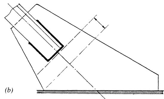
Fig. 11. Plastic hinge and free length of gusset plate
