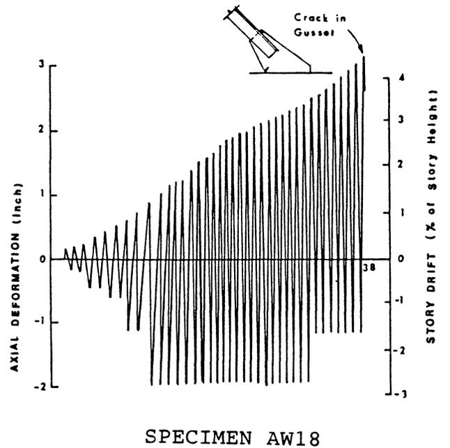
Fig. 5. Behavior of out-of-plane buckling specimens designed by modified procedure
