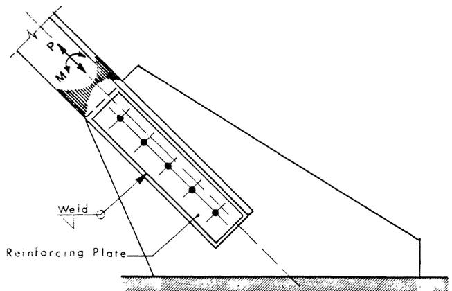
Fig. 9. Reinforcement of net section
