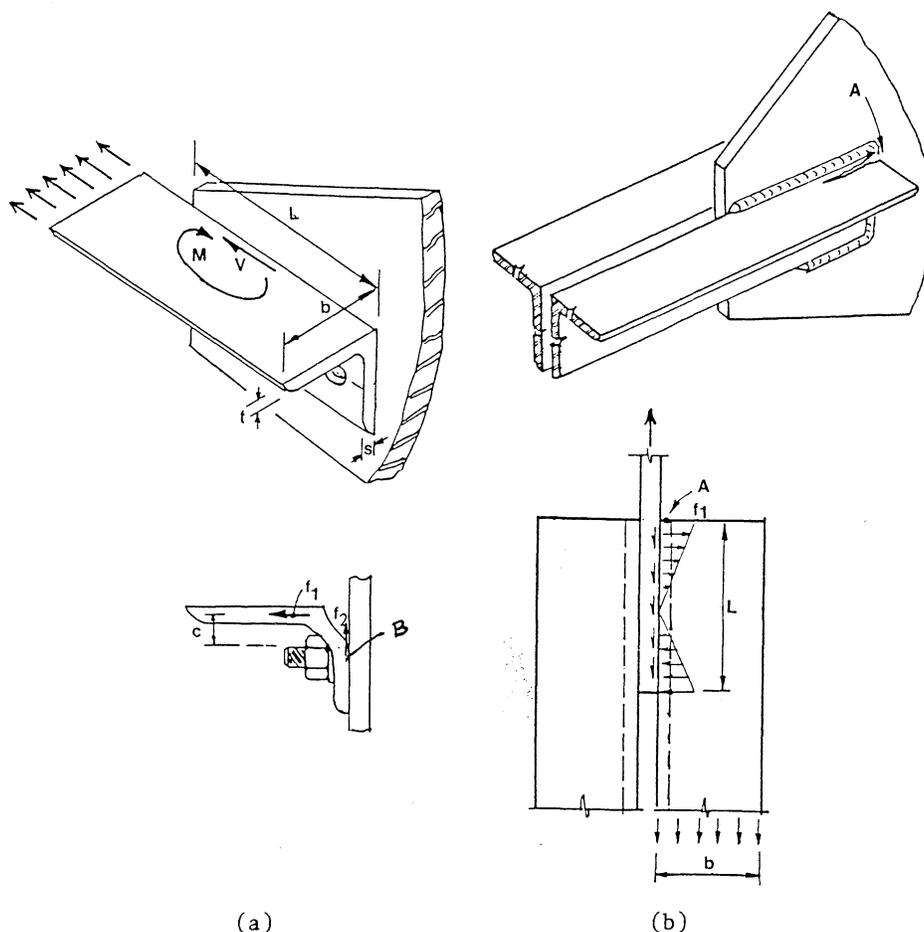
Fig. 8. Behavior of welded and bolted connections
