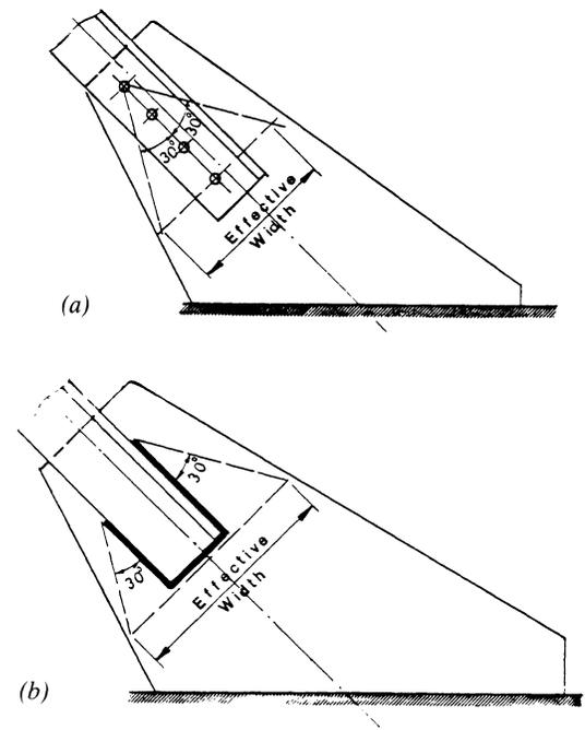
Fig.10. Effective width of gusset plate in bolted and welded connections
