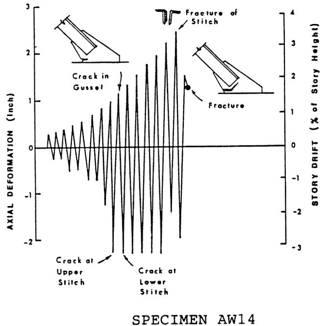
Fig. 4. Behavior of out-of-plane buckling specimens designed by AISC (1978) Specification
