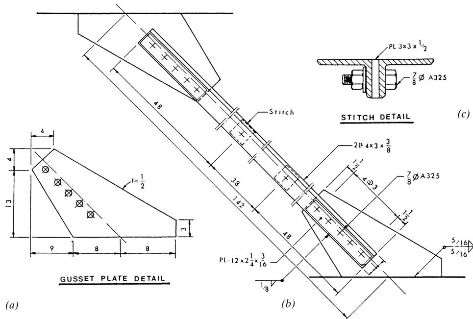
Fig. 13. Details of connections in Example 1
