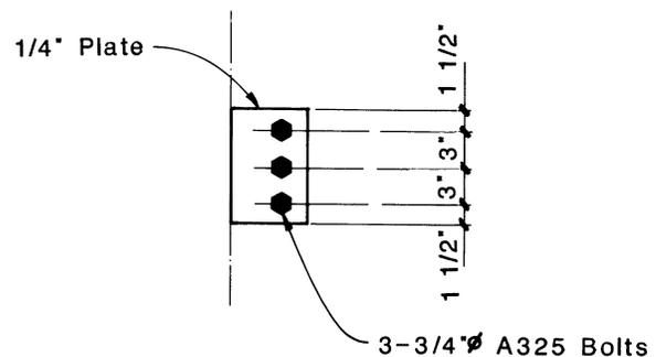
Fig. 10. Typical shear tab
