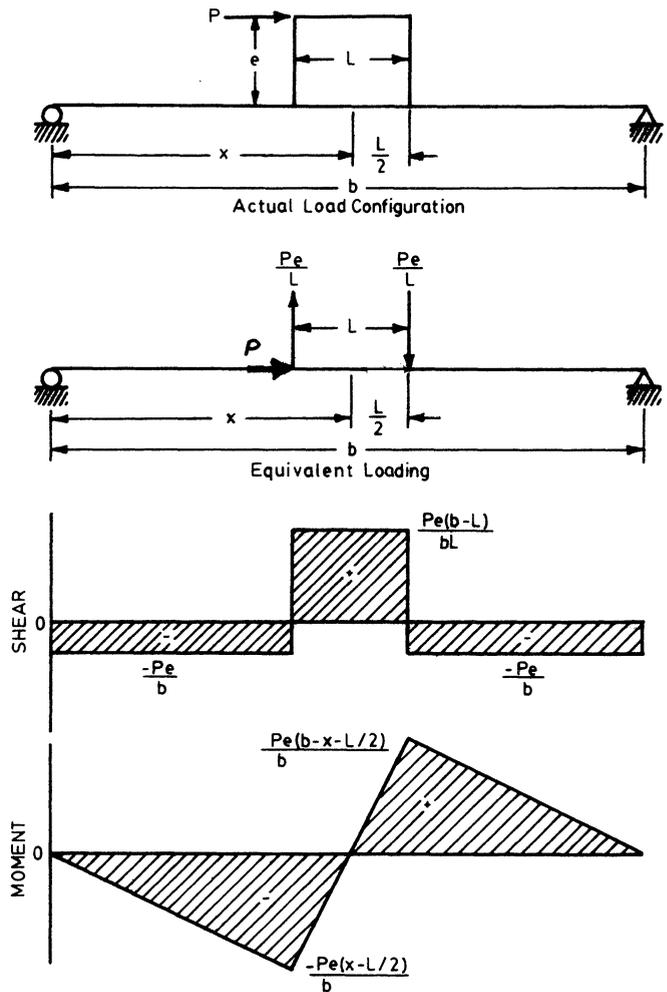
Fig. 8. Simplified equivalent loading
