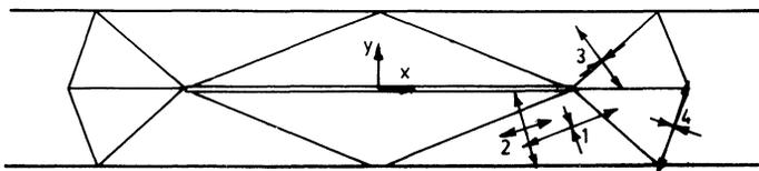
Fig. 5. Typical yield line pattern with principal directions of measured strain superimposed
