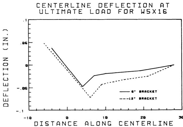
Fig. 10. Deflections along centerline of web at ultimate load for section exhibiting web failure
