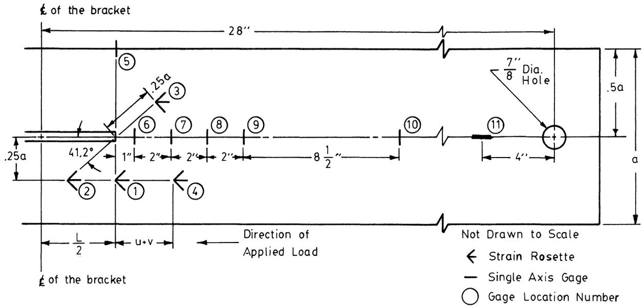
Fig. 3. Strain gage locations
