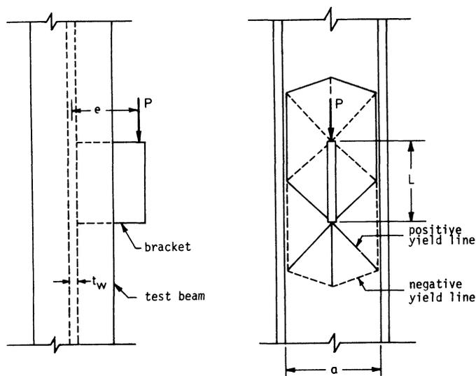
Fig. 1. Typical bracket connection and its yield line pattern at failure (Ref. 1).
