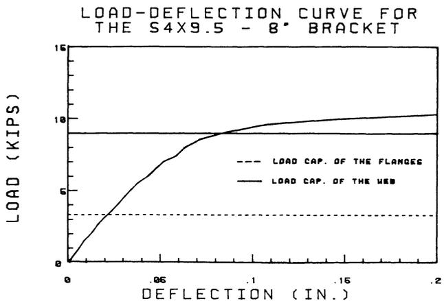
Fig. 14. Plot of load vs. maximum deflection of web for S4x9.5 section with 8-in. bracket
