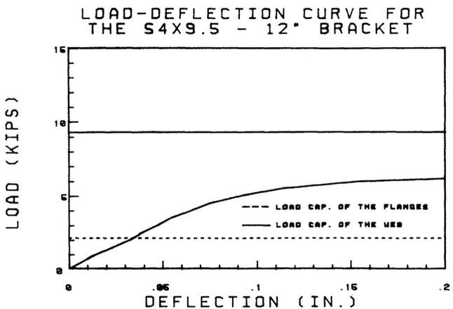
Fig. 15. Plot of load vs. maximum deflection of web for S4x9.5 section with 12-in. bracket
