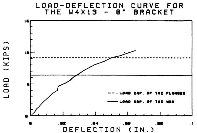
Fig. 12. Plot of load versus maximum deflection of web for W4×13 section with 8-in. bracket
