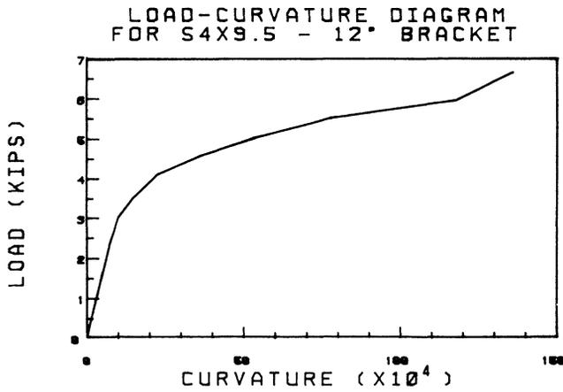
Fig. 9. Load-curvature diagram for S4×9.5 section with 12-in. bracket
