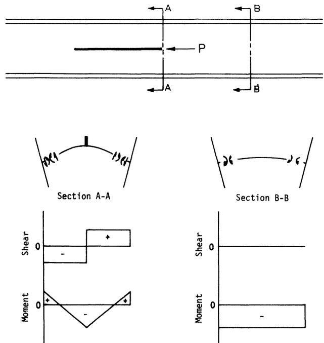
Fig. 6. Typical cross sections showing internal forces at failure
