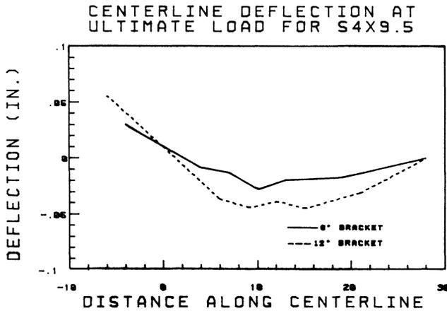
Fig. 11. Deflections along centerline of the web of section exhibiting flange failure
