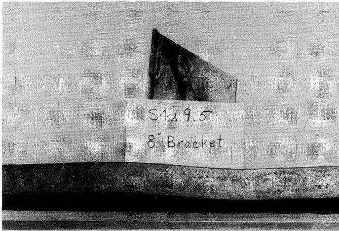
Fig. 7. Flange failure of the  $S4 \times 9.5$  sections
