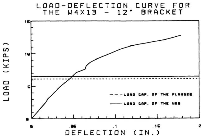
Fig. 13. Plot of load vs. maximum deflection of web for W4x13 section with 12-in. bracket
