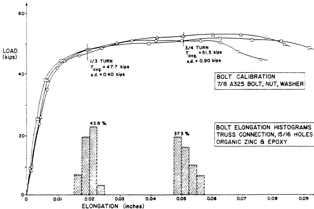
Fig. 9. Bolt force histograms and calibrations (1 kip = 4.45 kN, 1 in. = 25.4 mm)
