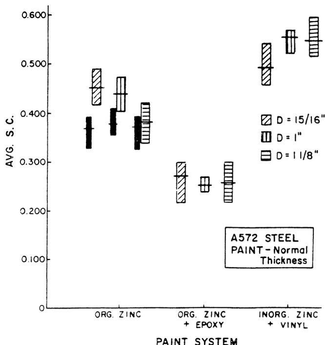
Fig. 7. Comparison of average slip coefficient for different hole sizes (1 in. = 25.4 mm)
