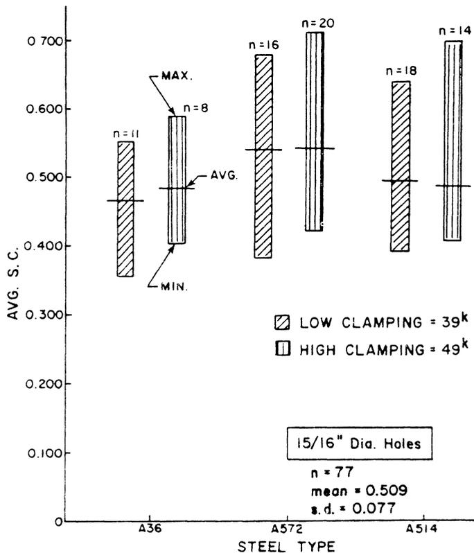
Fig. 4. Effect of steel type and clamping force, sandblasted surfaces (1 kip = 4.45 kN, 1 in. = 25.4 mm)
