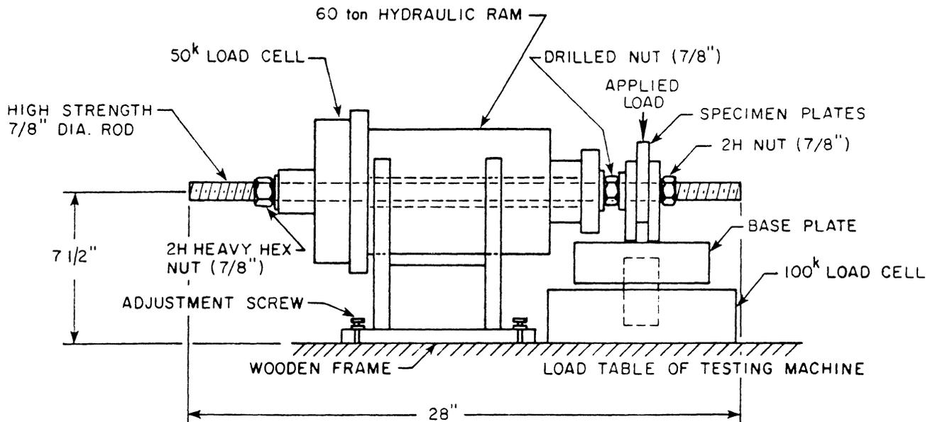
Fig. 1. Test setup schematic (1 in. = 25.4 mm)
