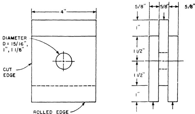
Fig. 2. Slip test specimen (1 in. = 25.4 mm)
