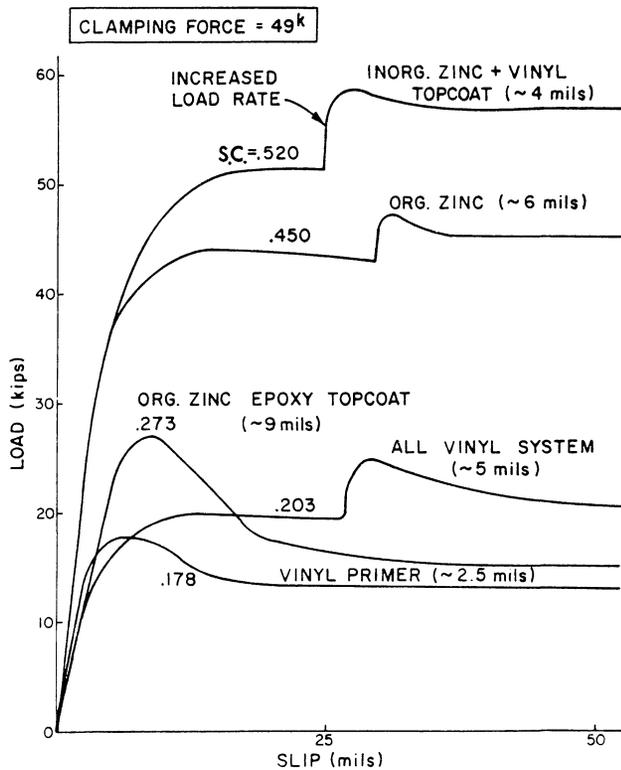
Fig. 5. Typical load-slip curves (1 kip = 4.45 kN)
