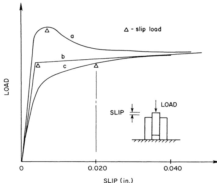
Fig. 3. Definition of slip load
