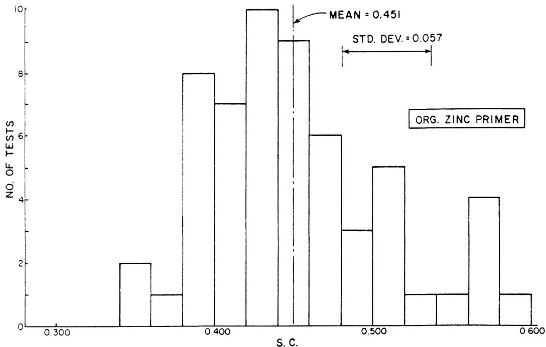
Fig. 6. Frequency distribution for organic zinc-rich coated A572 surfaces (58 tests)
