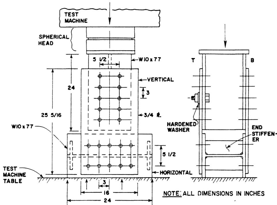
Fig. 8. Full-size slip connection (1 in. = 25.4 mm)
