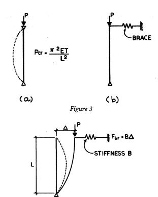
The stability of the column can be determined by displacing the column and then checking equilibrium of the deformed column. Thus, taking moments about the column base:
