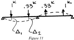
placed at an interior location in combination with 3-kip loads at the end diagonals; however, mathematically, the stiffness can be found from the deflection at the  $\frac{1}{3}$ -kip location.
