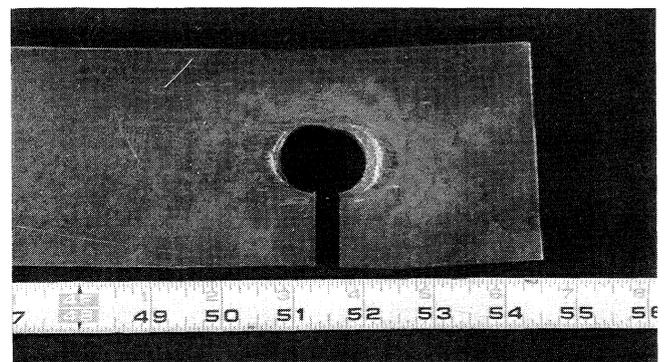
Fig. 17. Test sample area from which metallographic specimen was removed
