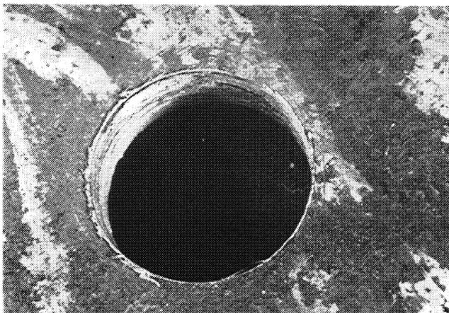
*Fig. 4. Hole in Sample P7 made by sub-punching and reaming to size*
