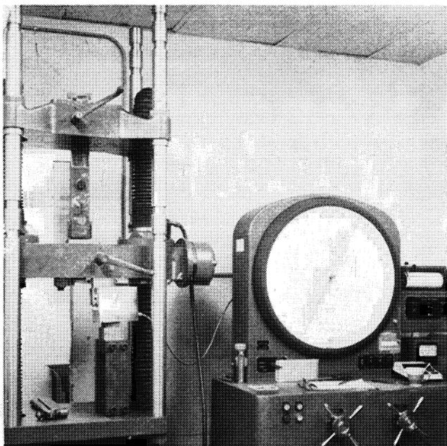
Fig. 1. Illustration of test apparatus used to test 18 specimens. Specimen (upper left) is bolted to fixture
