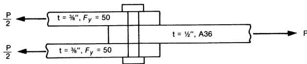
Fig. 8. Double-lap joint
