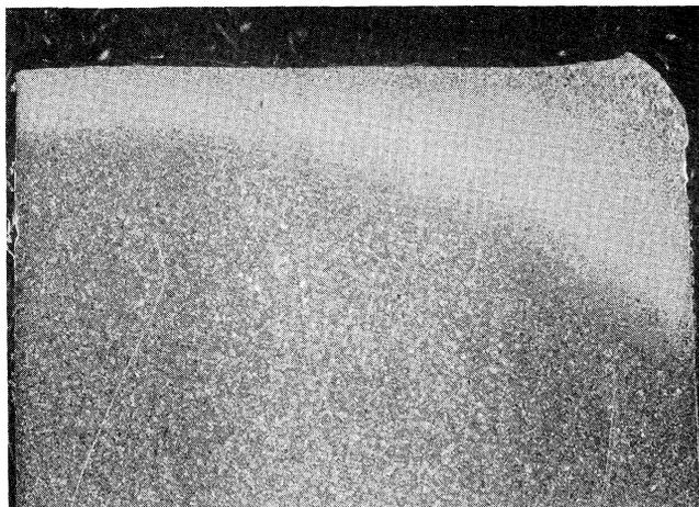
Fig. 19. Example of macro appearance of section from Sample P16. Magnification: 8X. Etchant: 1% Nital
