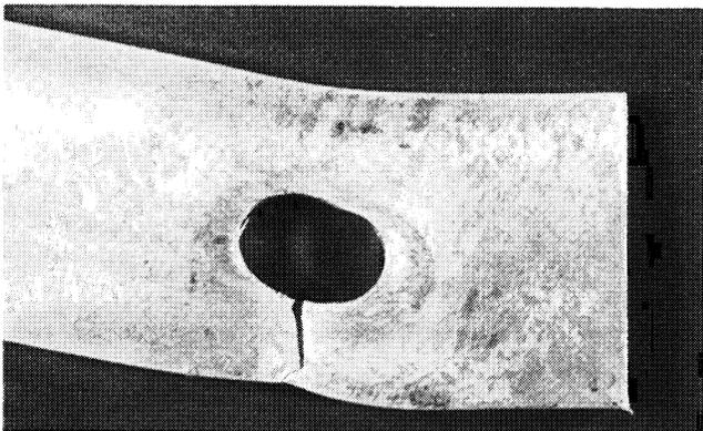
*Fig. 12. Hole in Sample P10 after testing, made by drilling*
