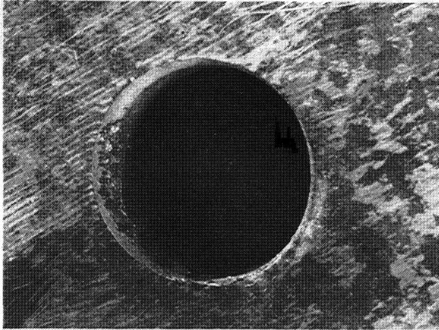
*Fig. 2. Hole in Sample P3 made by punching*
