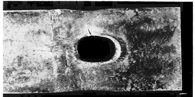
*Fig. 14. Hole in Sample P18 after testing, made by flame-cutting*
