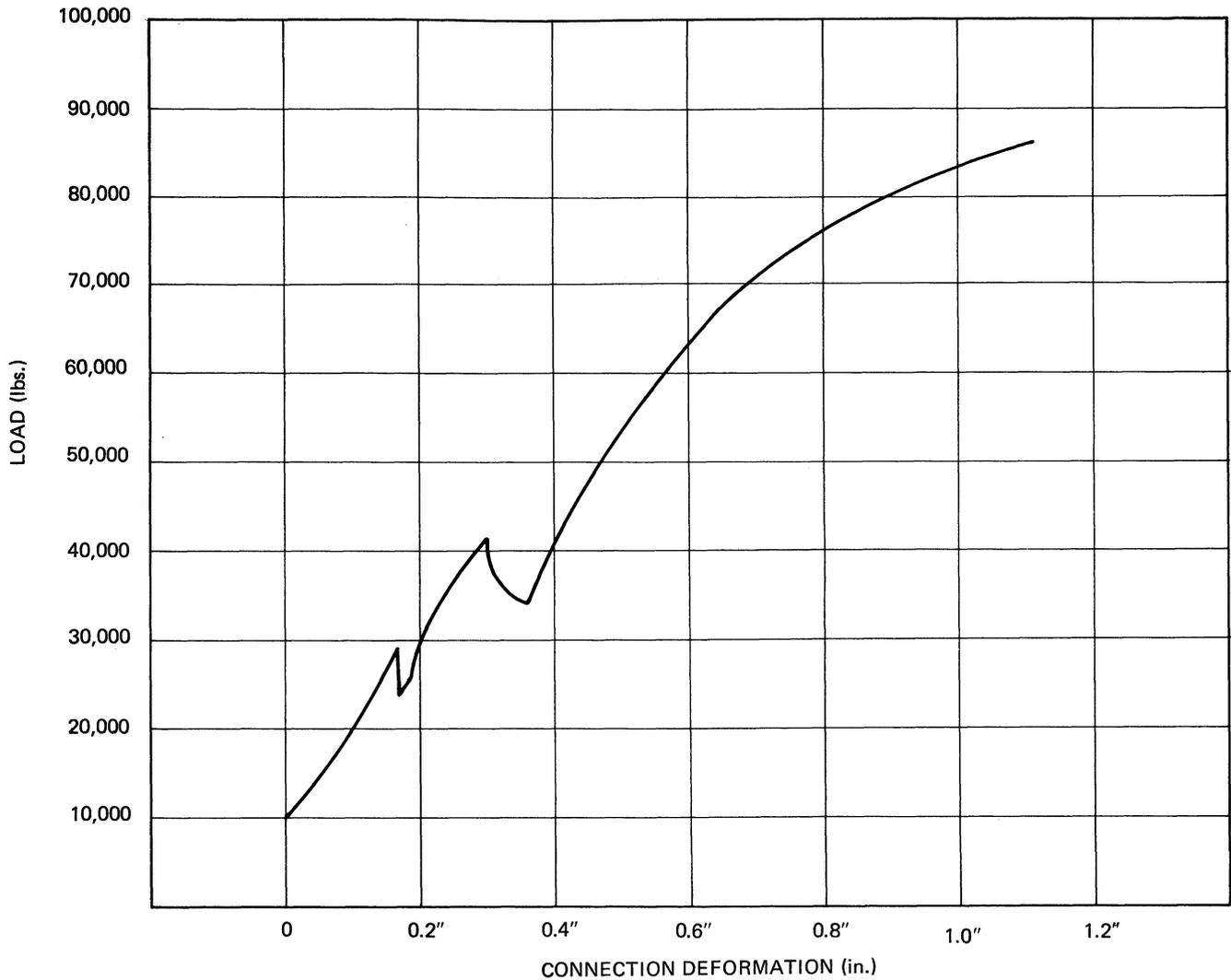
Fig. 16. Typical load-deformation relationship for a single joint, Sample P17
