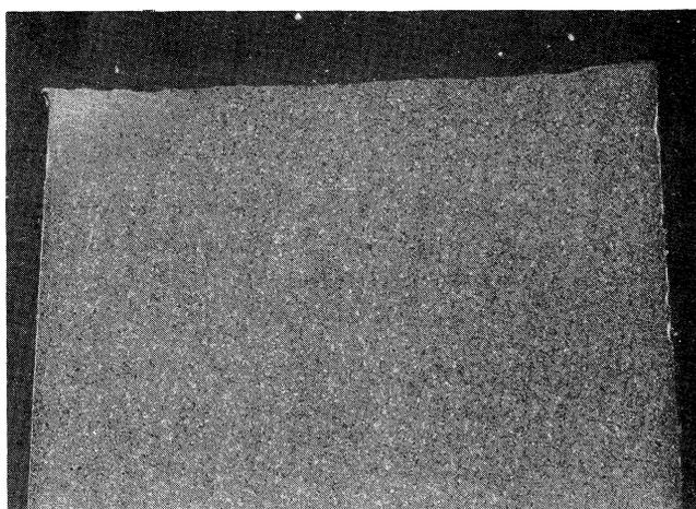
Fig. 18. Typical example of macro appearance of section from Sample P13. Small area of partial spheroidization at upper left. Magnification: 8X. Etchant: 1% Nital
