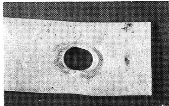
Fig. 10. Hole in Sample P5 after testing, made by punching and grinding burrs
