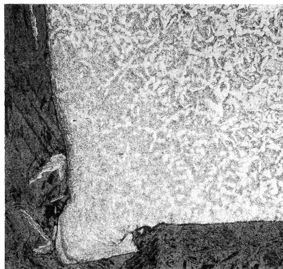
Fig. 20. Partial spheroidization at corner of Sample P15. Magnification: 100X. Etchant: 1% Nital
