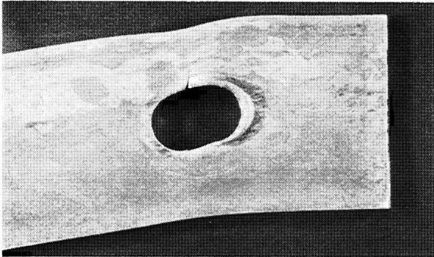
*Fig. 11. Hole in Sample P7 after testing, made by sub-punching and reaming*
