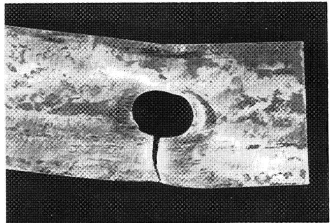
Fig. 9. Hole in Sample P3 after testing, initially made by punching
