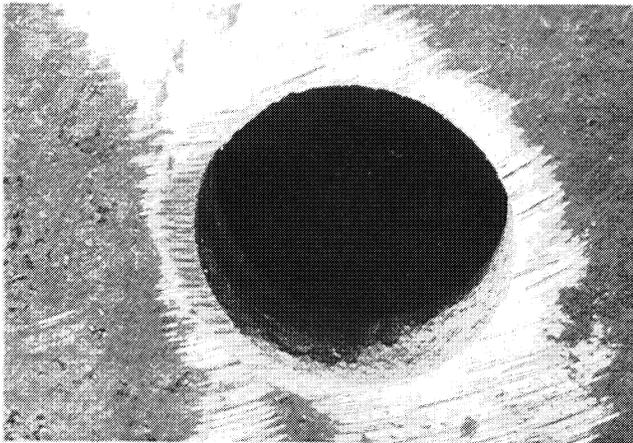
*Fig. 3. Hole in Sample P5 made by punching and grinding off burrs*
