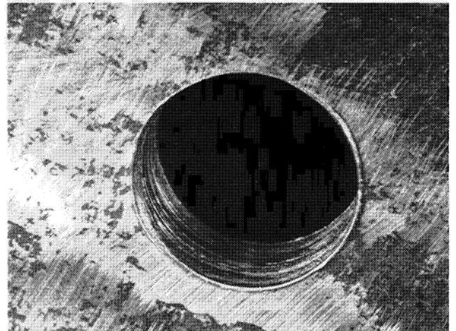
*Fig. 5. Hole in Sample P10 made by drilling*
