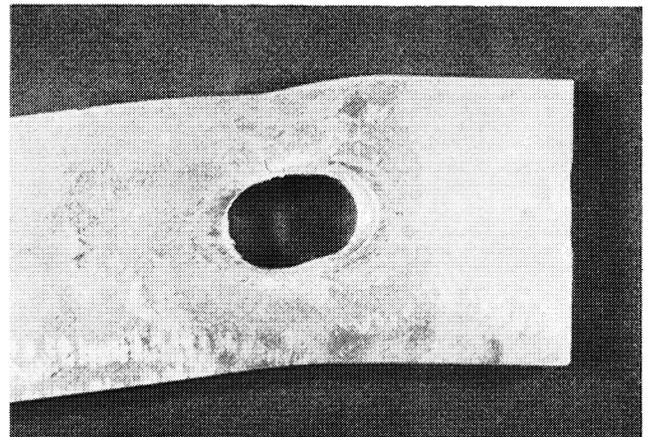
*Fig. 13. Hole in Sample P15 after testing, made by flame-cutting and reaming*
