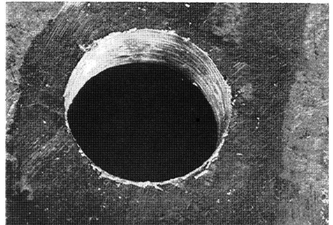
*Fig. 6. Hole in Sample P15 made by flame-cutting and reaming to size*
