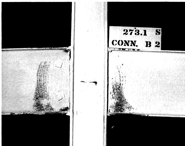
Fig. 22. Interior beam-to-column connection with plastic hinge in both beams
