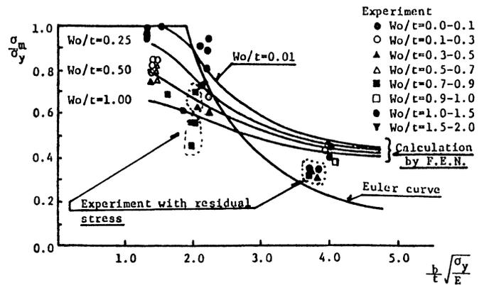
Fig. J4.1. Ultimate strength of square plates subjected to compression
