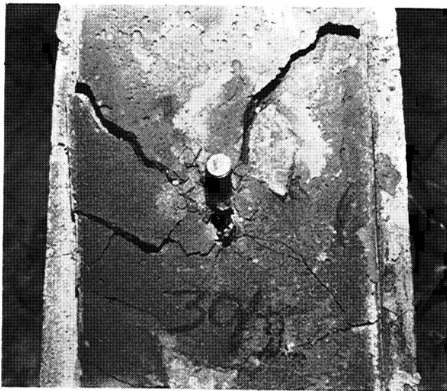
Fig. 3. Grout failure; load applied at 30°
