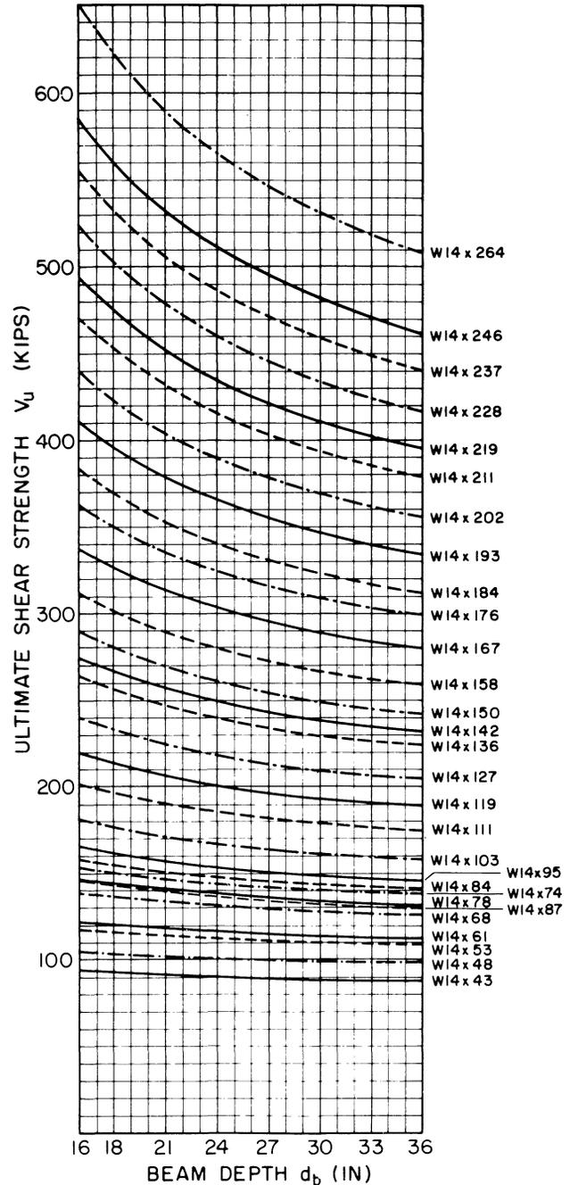
Fig. 9. Ultimate shear strength for unreinforced joints in W14 columns of A36 steel
