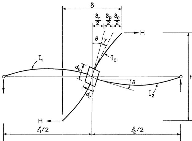
Fig. 10. Components of lateral deflection in beam-column assembly
