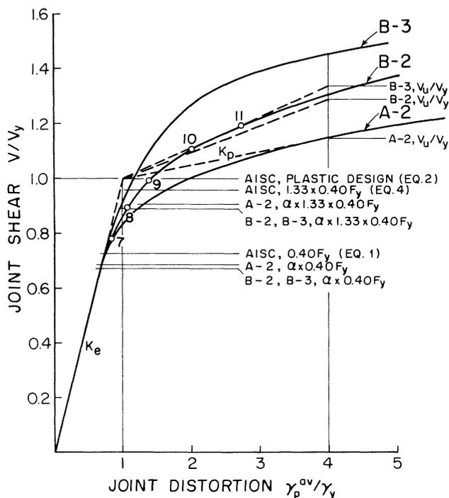
Fig. 5. Shear force-distortion diagrams for joints
