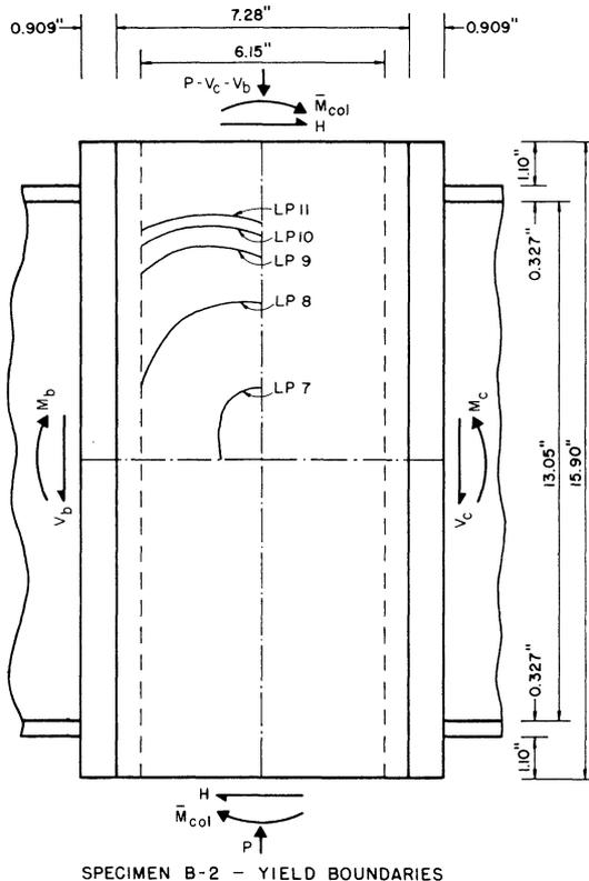
Fig. 6. Propagation of yield boundary in panel
