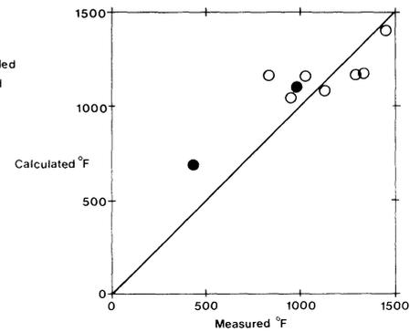
Fig. 25. Measured and calculated temperatures of spandrel beam, from large-scale tests with forced draft, Underwriters' Laboratories (Note: Shield is 2-ft awning)
