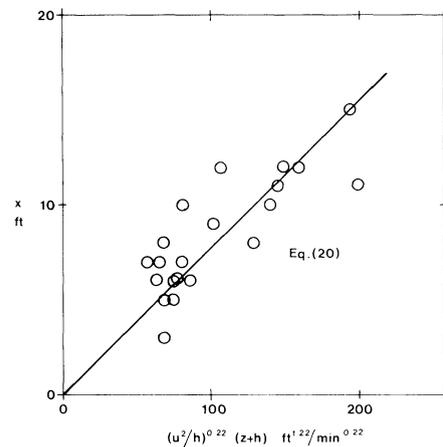
Fig. 10. Horizontal projection of flame tip for large-scale tests with forced draft, Underwriters' Laboratories data (Note: Range of  $u^2/h$ : 1000-22,500 ft/min<sup>2</sup>)
