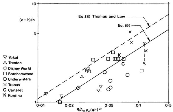
Fig. 7. Flame heights for large-scale tests with natural draft (Note: Range of  $n$ : 0.5-18.7)
