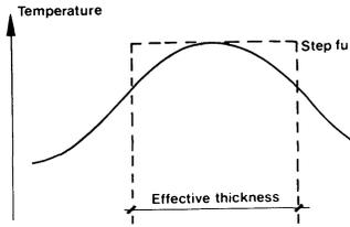
Fig. 12. Temperature distribution across flame section
