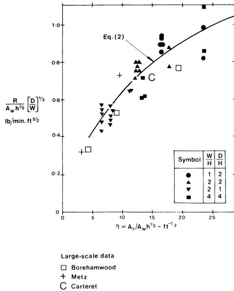
Fig. 2. Variation of  $R/A_w h^{1/2}$  with compartment size and ventilation, as given by Thomas for CIB data
