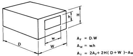
Fig. 1. Simple fire compartment
