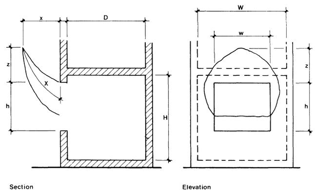
Fig. 6. Dimensions used in calculations of flame projection
