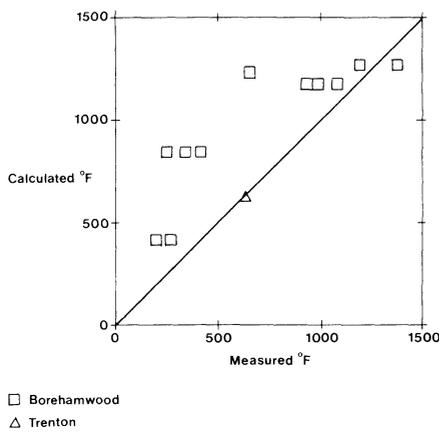
Fig. 22. Measured and calculated temperatures of spandrel beams engulfed in flame, from large-scale tests with natural draft
