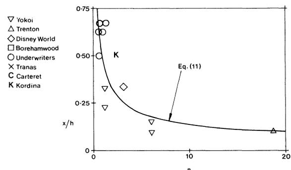
Fig. 8. Horizontal projection of flame tip for large-scale tests with natural draft, wall above
