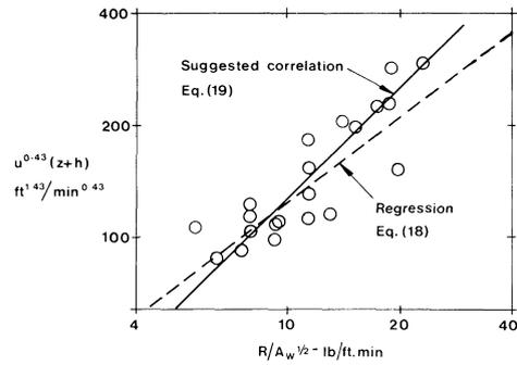
Fig. 9. Flame heights for large-scale tests with forced draft, Underwriters' Laboratories data (Note: Range of  $f$ : 100-367 ft/min)
