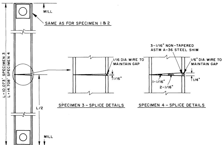
Fig. 2. Details of Specimens No. 3 and No. 4
