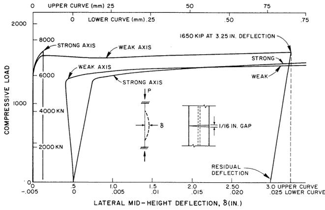
Fig. 6. Load-deflection for Specimen No. 1
