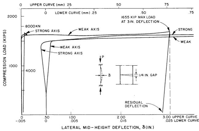
Fig. 7. Load-deflection for Specimen No. 2
