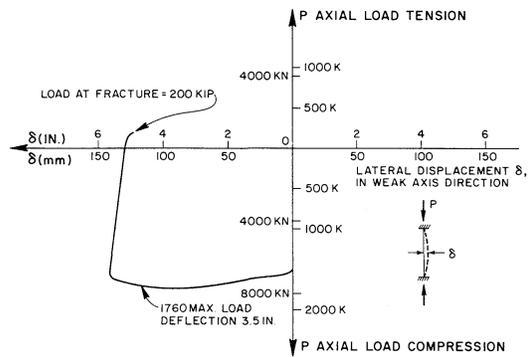
Fig. 16. Load-deflection hysteresis for Specimen No. 4
