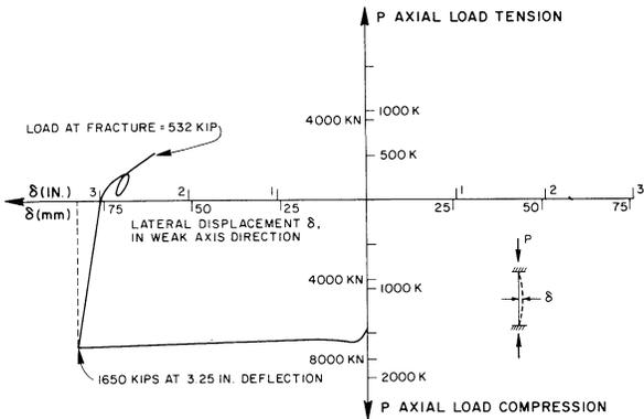
Fig. 13. Load-deflection hysteresis for Specimen No. 1
