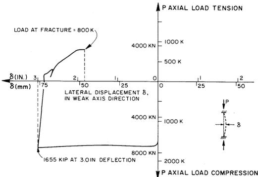
Fig. 14. Load-deflection hysteresis for Specimen No. 2
