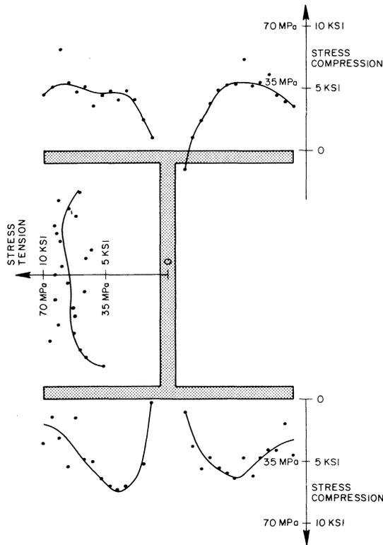
Fig. 4. Results of residual stress measurements
