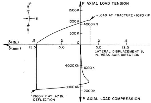
Fig. 15. Load-deflection hysteresis for Specimen No. 3
