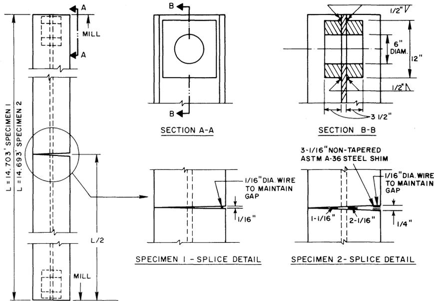
Fig. 1. Details of Specimens No. 1 and No. 2
