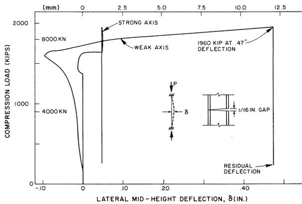
Fig. 8. Load-deflection for Specimen No. 3
