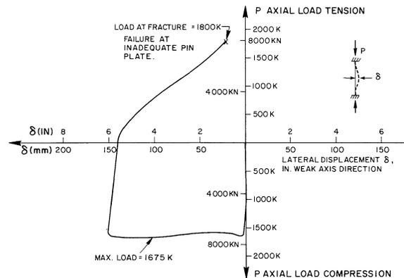
Fig. 17. Load-deflection hysteresis for Specimen No. 5
