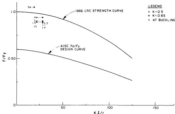
Fig. 18. Theoretical and experimental column strengths
