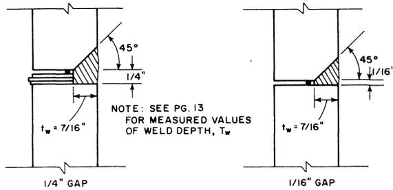
Fig. 3. Flange weld detail of splice
