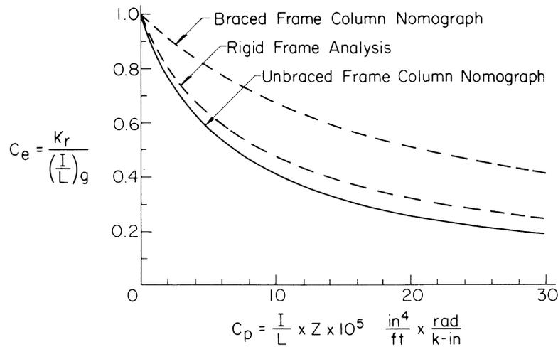
Fig. 2. Chart for determination of  $K_r$ .
