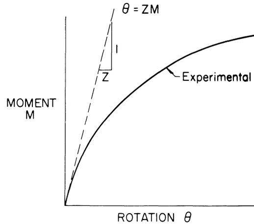
Fig. 4. Typical moment rotation curve of semi-rigid connection
