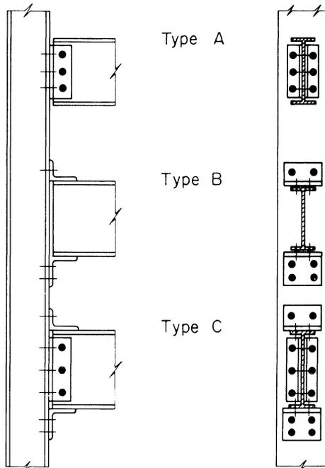
Fig. 3. Three types of semi-rigid connections
