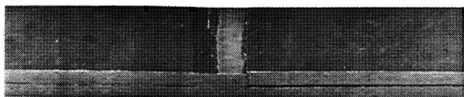
Fig. 11. Typical failure of welded specimen with discontinuity
